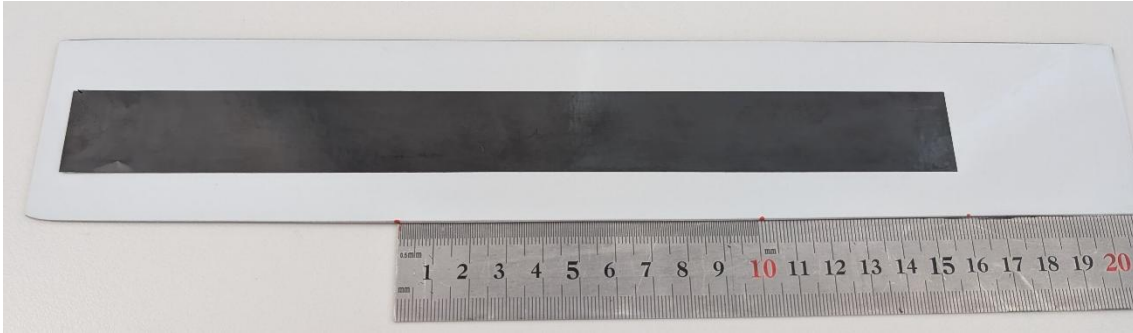
Figure 7: Tape Application, Insulation Tape
