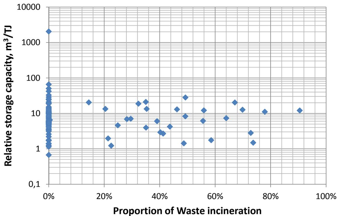
Diagram 8 - The relative storage capacity for all analyzed systems with installed storage capacity, compared with their proportion of heat generated by waste incineration.
