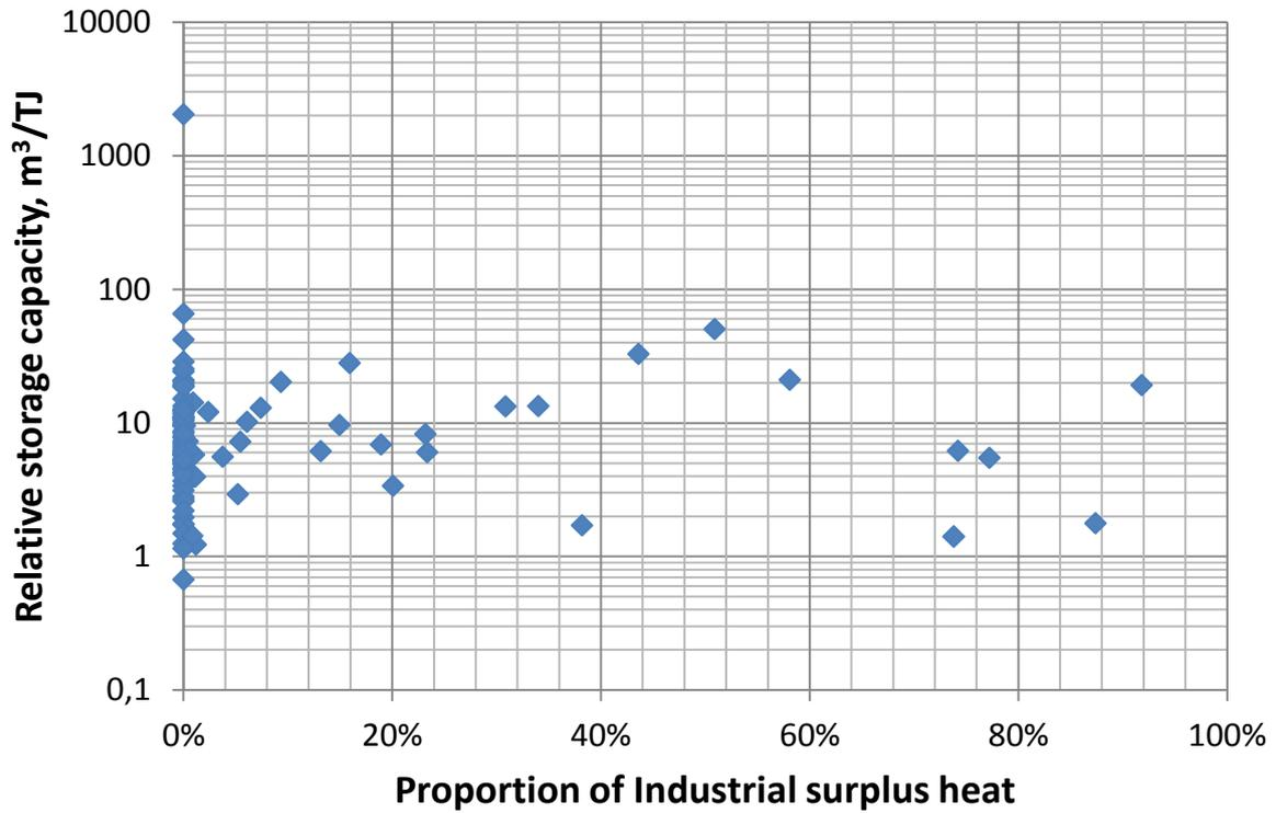
Diagram 10 - The relative storage capacity for all analyzed systems with installed storage capacity, compared with their proportion of heat generated from industrial surplus heat.
