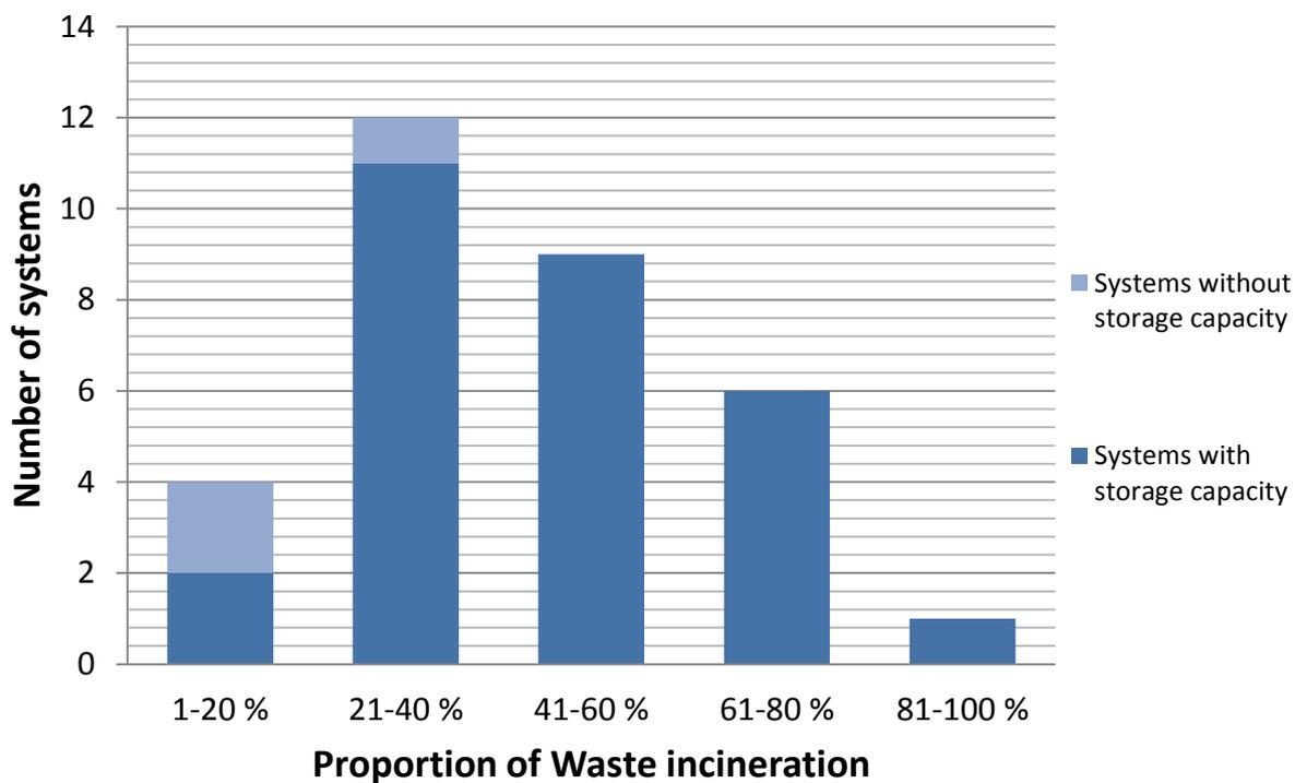
Diagram 9 - The number of analyzed systems that utilizes waste incineration for heat generation are compared in order to investigate the proportion that have installed heat storage capacity.
