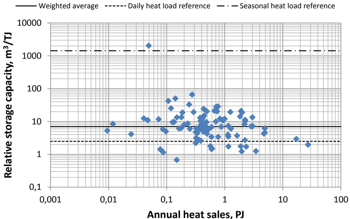
**Diagram 3 - The relative storage capacity for each system with installed heat storages, compared to the systems annual heat sales.**
