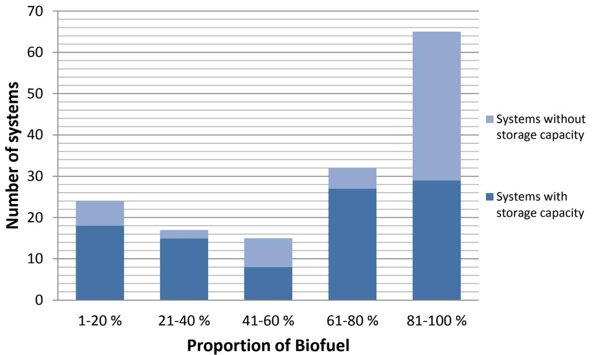
Diagram 7 - The number of analyzed systems that utilizes biofuel for heat generation are compared in order to investigate the proportion that have installed heat storage capacity.
