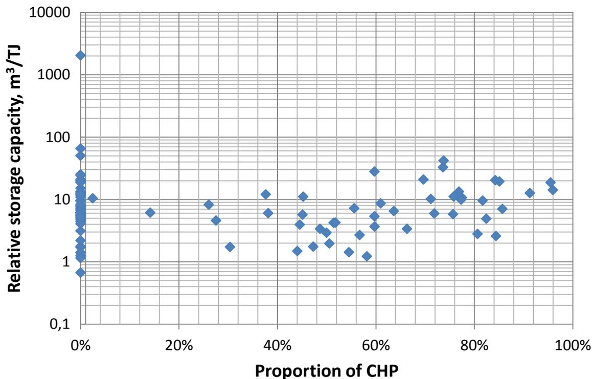
Diagram 4 - The relative storage capacity for all analyzed systems with installed storage capacity, compared with their proportion of heat generated in CHP plants.
