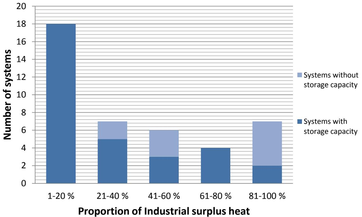
Diagram 11 - The number of analyzed systems that utilizes industrial surplus heat are compared in order to investigate the proportion that have installed heat storage capacity.
