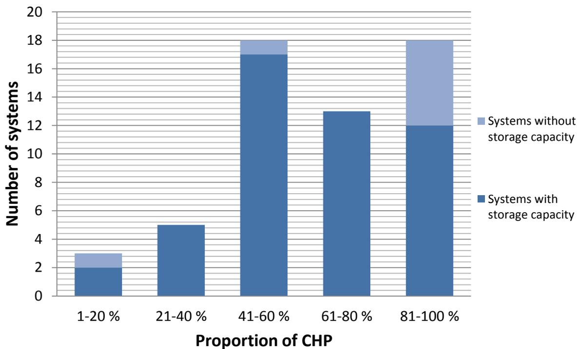
Diagram 5 - The number of analyzed systems that utilizes CHP plants for heat generation are compared in order to investigate the proportion that have installed heat storage capacity.
