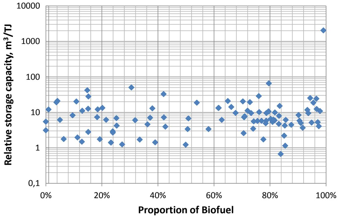
Diagram 6 - The relative storage capacity for all analyzed systems with installed storage capacity, compared with their proportion of heat generated from biofuel.
