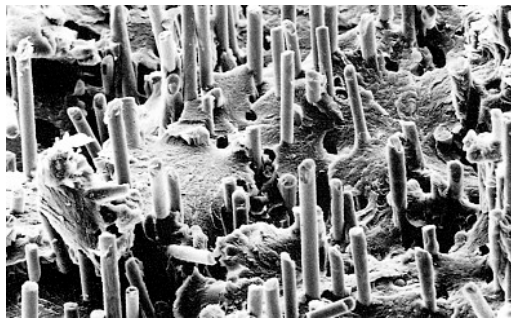
Figur 3.2 Brottytan i fiberkomposit [11]
