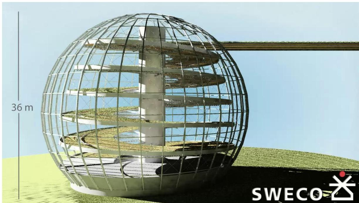
Fig 1: Illustration of Plantagon, Linköping. Globular helix design with internal rotating structure
