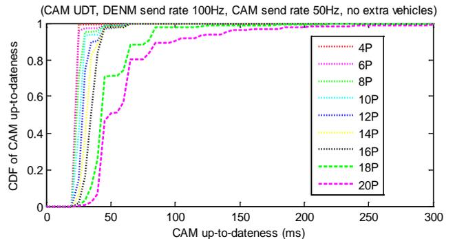
Figure. 13: CAM UTD with coexisting DENM traffic on the control channel (platoon vehicles only)
