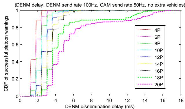
Figure. 10: CC - DENM DD with no extra vehicles and for CAM send rate 50 Hz
