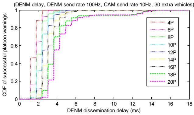
Figure 5: CC - DENM DD with 30 extra vehicles and for CAM send rate 10 Hz
