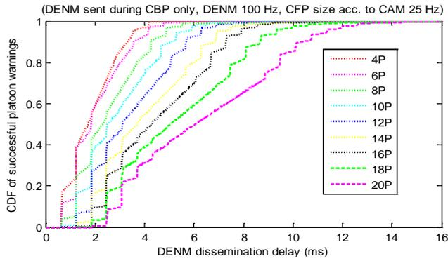
Figure 6: SC - DENM DD, based on full CBT size and CFP for CAM send rate 25 Hz
