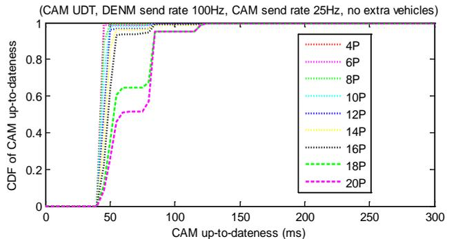
Figure. 12: CAM UTD with coexisting DENM traffic on the control channel (platoon vehicles only)
