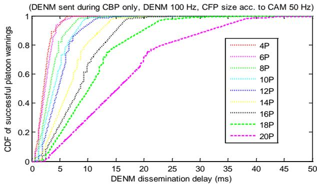
Figure.9: SC - DENM DD, based on half CBT size and CFP for CAM send rate 50 Hz
