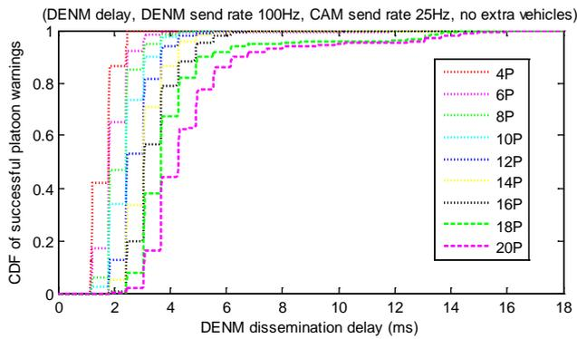
Figure 7: CC - DENM DD with no extra vehicles and for CAM send rate 25 Hz
