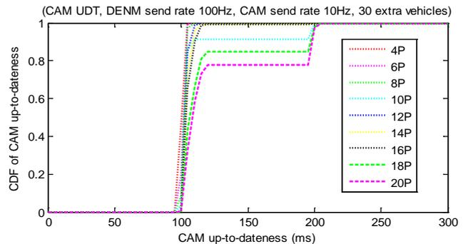
Figure. 11: CAM UTD with coexisting DENM traffic on the control channel (platoon and non-platoon vehicles)
