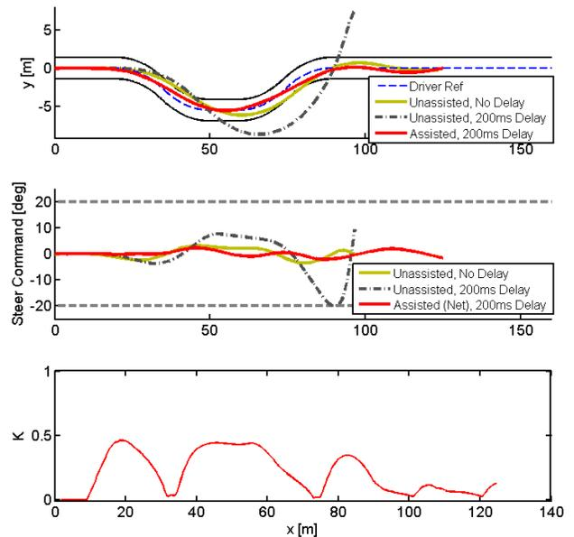
**Figure 8. Simulation results illustrating the effect of a 200ms time delay on the driver model and demonstrating the ability of the semi-autonomous framework to assist the driver**
