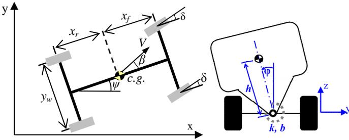
Figure 2. Vehicle model used in MPC controller
