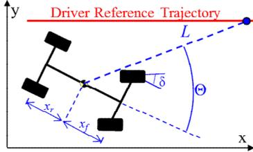
Figure 5. Driver model parameter illustration
