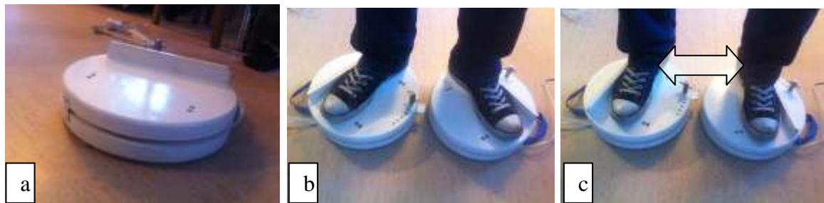
**Figure 1.** (a) Side view of the device,  $\varnothing$  0.32 m, height 0.065 m. (b) Starting position with the feet against the supports, (c) By pushing the feet apart the top plates will rotate internally. The subject is in position to squat
