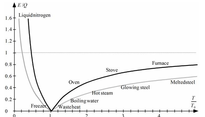
Fig. 1 Exergy factor ( $E/Q$ ) of heat and cold as a function of ratio of temperature to environment temperature.
