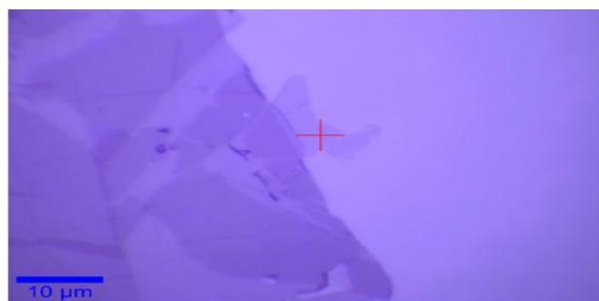
Fig3.4 - Bilayer graphene.
