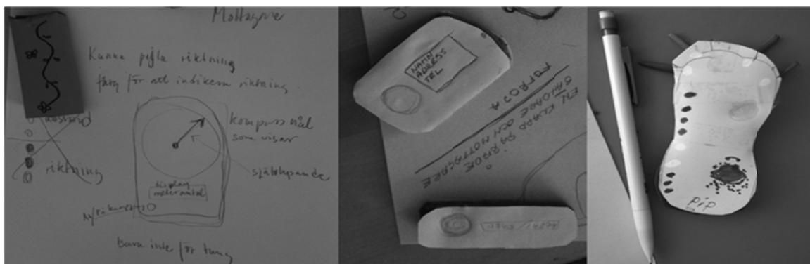
Fig 4. Left: a paper prototype of the receiver and the sender as inside a piece of jewellery. Middle the sender with a nametag and a button. Right a receiver made of paper, flower foam brick and flower sticks.
