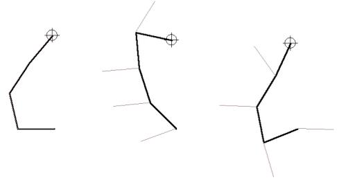
Fig. 2. Screenshots from the tutorials. The thick line is a planar robot arm, and the crosshair is the end-effector. The thin lines indicate desired “posture” positions for each joint. Here, the posture is projected into the nullspace of an end-effector position task.
