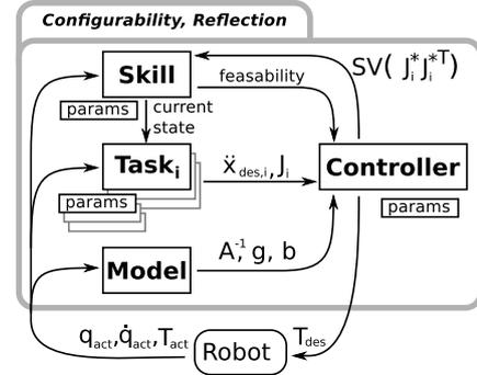
Fig. 1. Architectural overview of the Whole-Body Control software. SV stands for *singular values*,  $T_{des}$  is the desired joint-torque vector, and  $\{q_{act}, \dot{q}_{act}, T_{act}\}$  are the actual joint positions, velocities, and torques. The rest of the notation is the same as in Algorithm ??.
