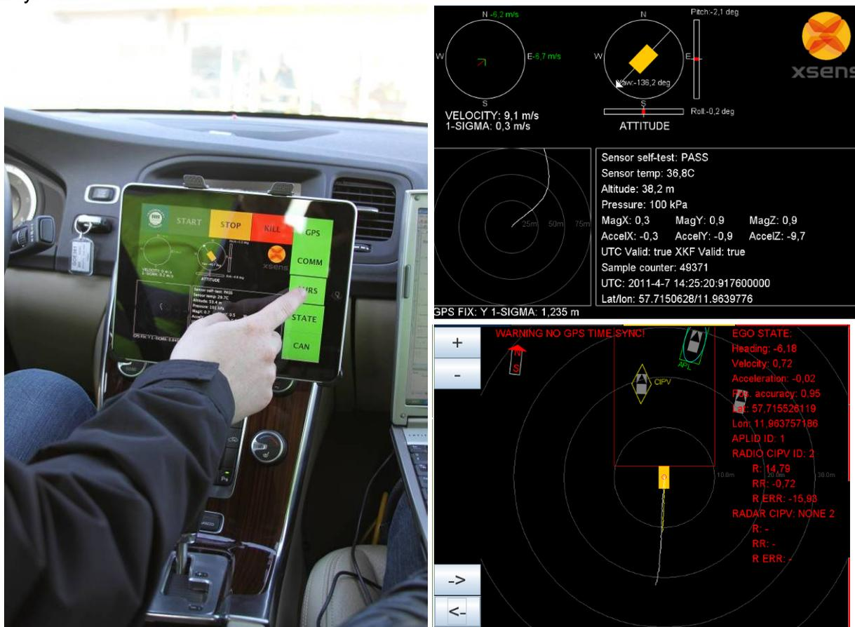
**Figure 10. Left, iPad used to display the HMI. Top right, AHRS HMI screenshot. Bottom right, state estimator HMI screenshot**
