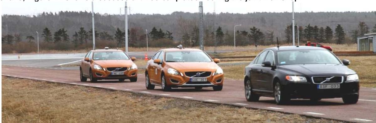
**Figure 11. Two actuated Volvo S60 following a non-actuated Volvo S80 lead vehicle during the joint CoAct testing workshop in March 2011.**
