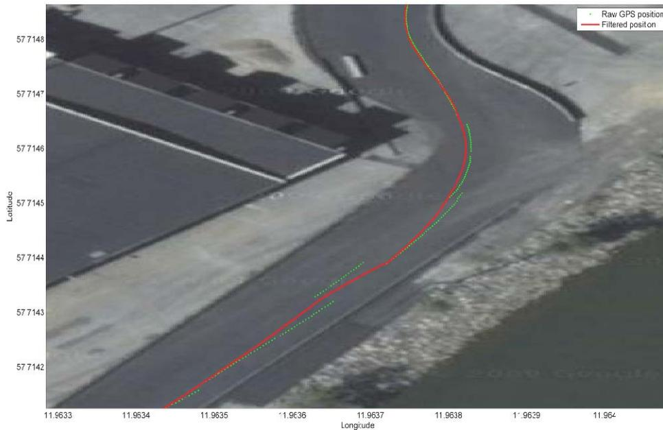
**Figure 4. GPS disturbances are handled by incorporating data from the CAN bus and from inertial sensors.**
