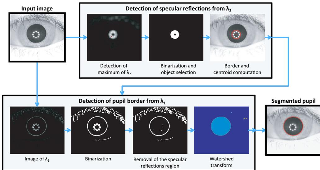
Fig. 3. System model for pupil detection/segmentation by Structure Tensor analysis.
