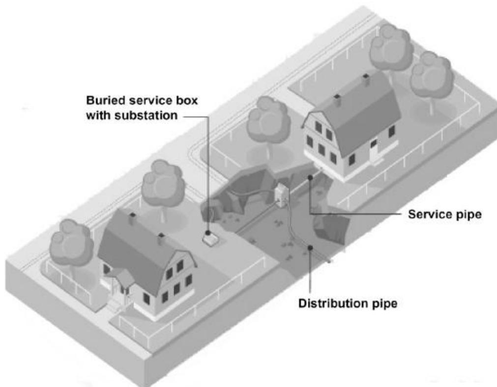
Figure 8. The Finnova system suggested as an innovative solution for district-heating distribution. It is based on joint-less flexible pipelines connecting underground sub-stations placed in cabinets buried at the plot boundary. Source [6], [11]
