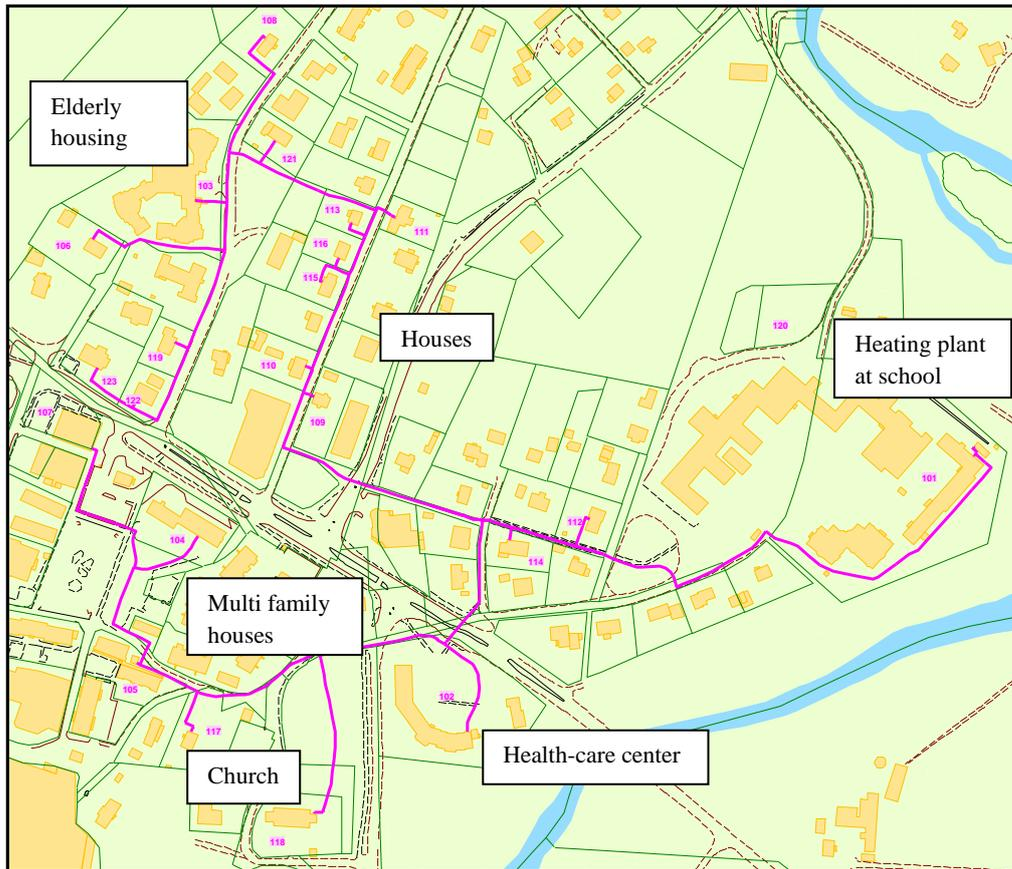
Figure 4. Map of distribution system of district heating System in Ullared.
