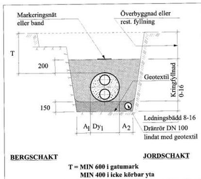
Figure 5. Section through pipe trench in Ullared.
