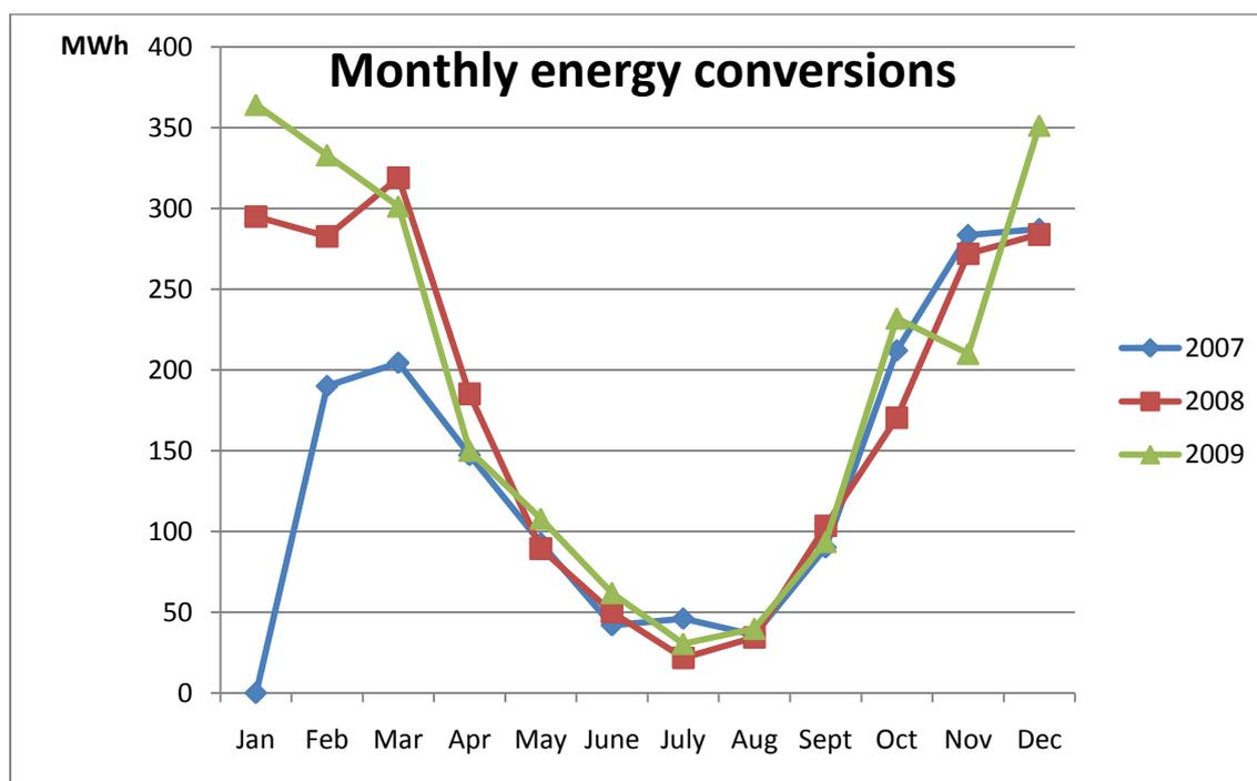
Figure 6. Outcome of converted energy/month by the heating plant in Ullared during 2007-2009. Note that the first metered figures are from February 2007 when the new heating plant became operational.
