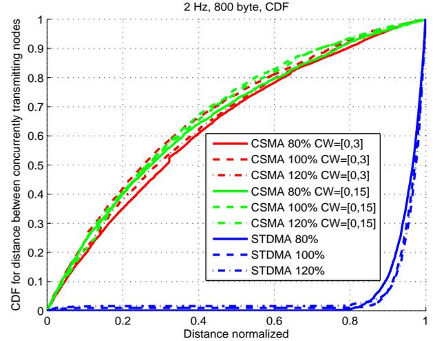
Figure 4. The CDF for the distance between concurrently transmitting nodes for 2 Hz and 800 byte packets.
