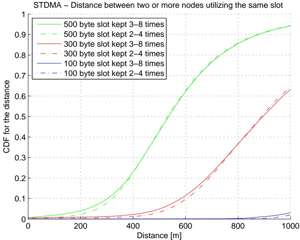
**Figure 5. STDMA: CDF for distance between two or more nodes using the same slot.**
