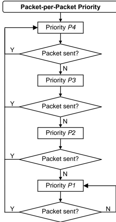
**Figure 1. New algorithm for changing the priority on a packet-per-packet basis.**
