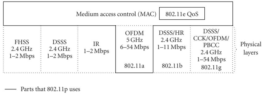
FIGURE 1: An overview of the WLAN family 802.11, showing in bold which parts that 802.11p will use and modify.
