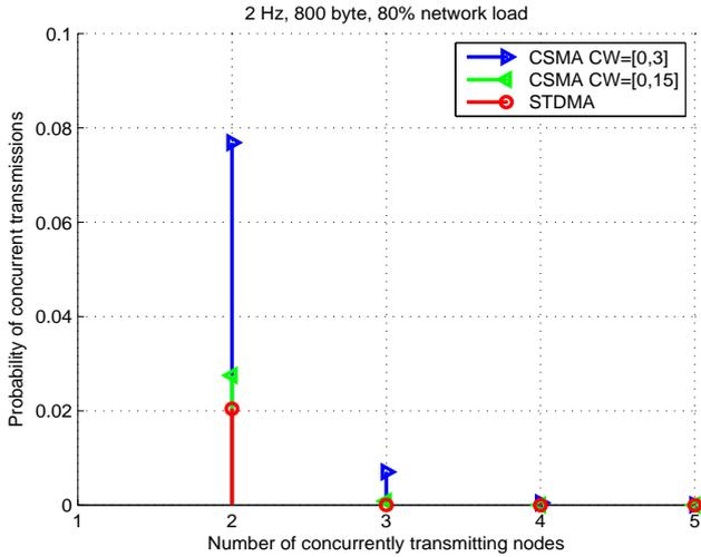
Figure 3. The probability that nodes transmit concurrently out of the number of *successful channel access requests* for 2 Hz and 800 byte at a network load of 80%.
