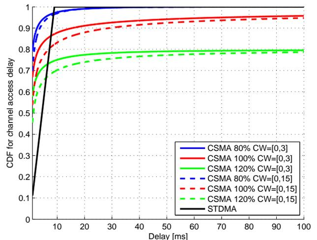
Figure 2. The CDF for channel access delay for CSMA and STDMA for 10 Hz and 300 byte at different traffic loads – 80%, 100% and 120%. The CSMA has also two different CW setting.
