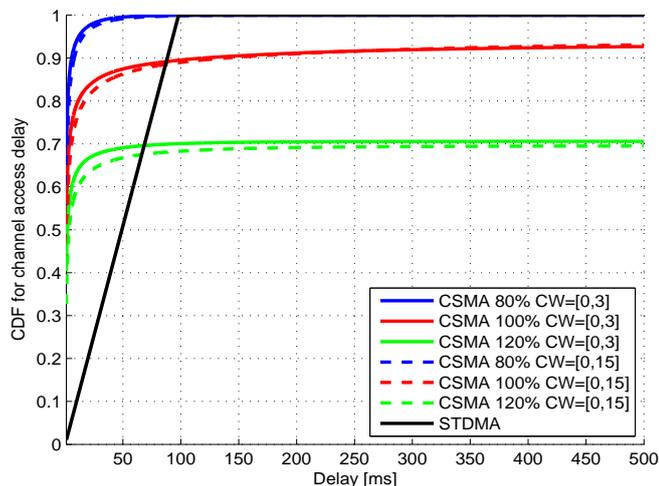
Figure 1. The CDF for channel access delay for CSMA and STDMA for 2 Hz and 800 byte at different traffic loads – 80%, 100% and 120%. The CSMA has also two different CW setting.
