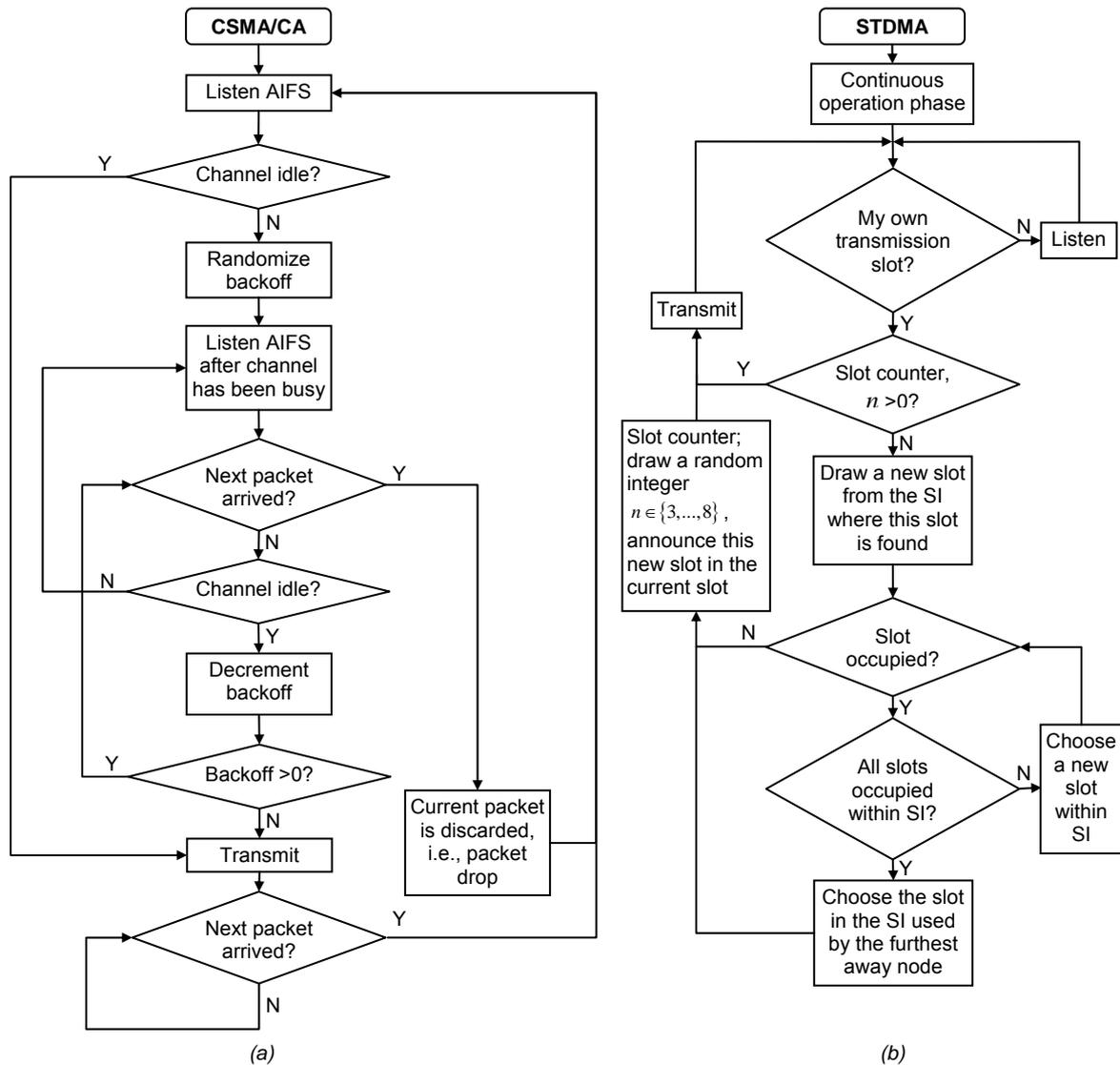
**Figure 1. The two MAC procedures examined in this thesis work using a data traffic model with broadcasted time-driven messages at predetermined heartbeat rates; (a) the CSMA procedure according to 802.11p and (b) continuous operation phase of STDMA**
