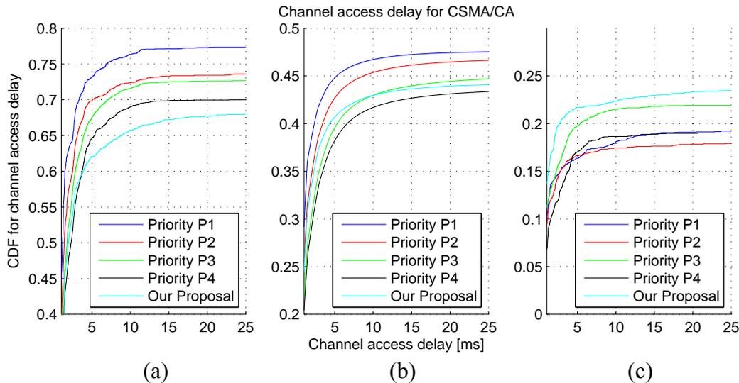
**Figure 4. CDF for the channel access delay in CSMA/CA for the different priorities and our proposed packet-per-packet priority change. (a) Best case for an individual node, (b) average case for all nodes and (c) worst case for an individual node.**
