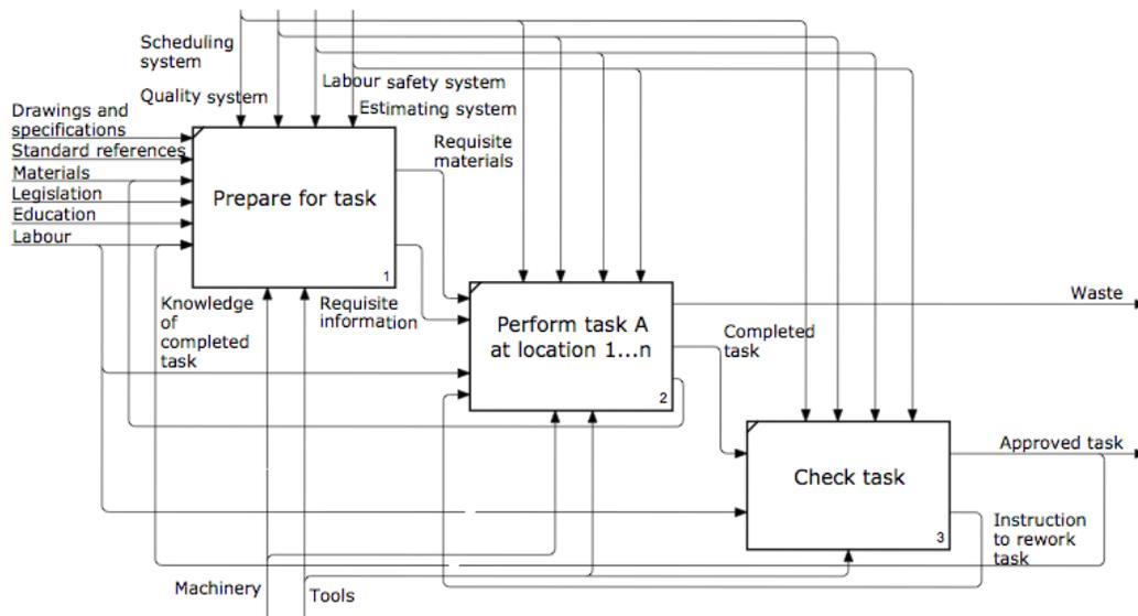
Figure. 1: A generic process model illustrating the flow of information and resources needed to perform Task A at location n on the construction site. (Adapted from CIB78 1997 by Persson & Hansson 2008)
