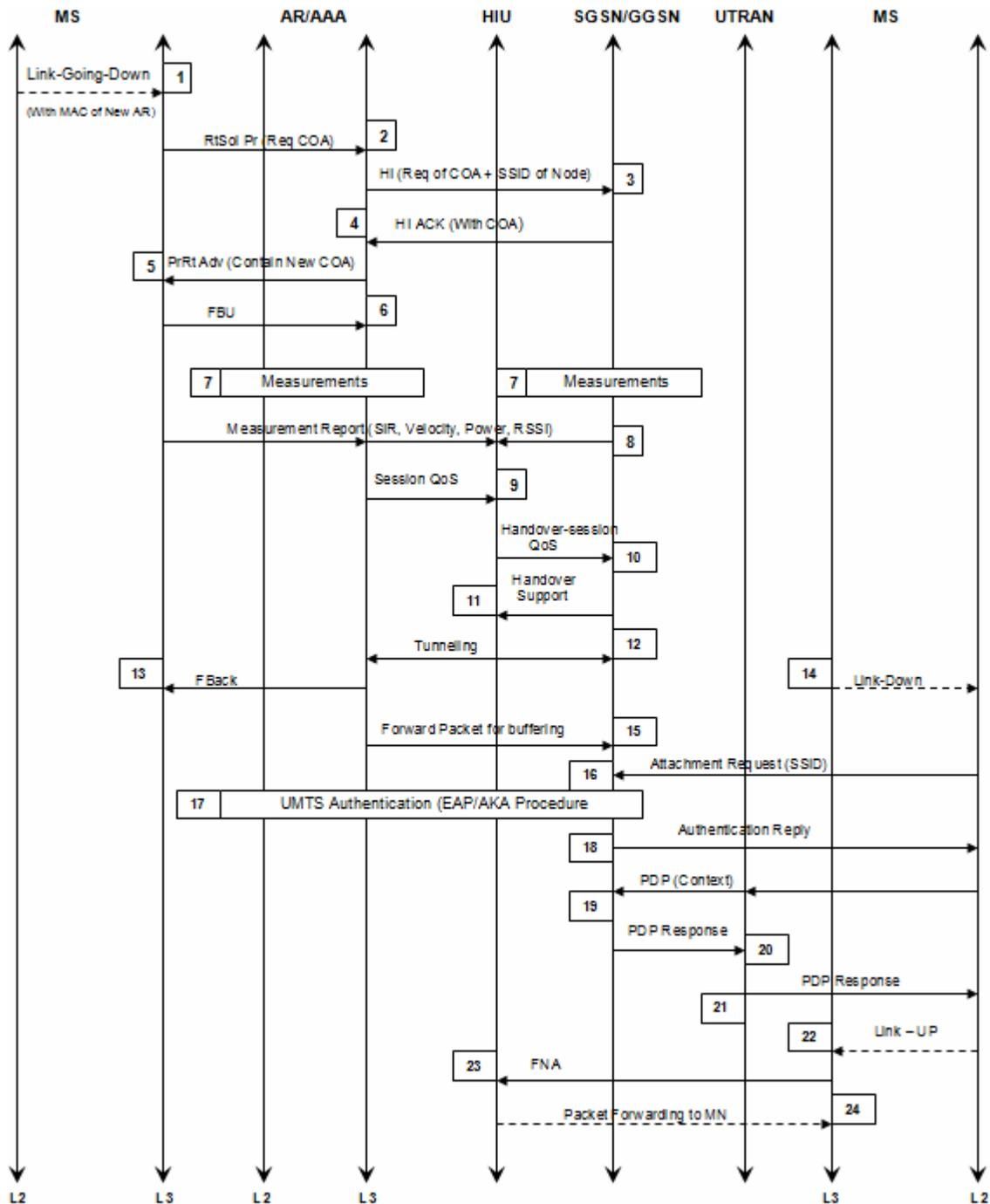
Figure 8.2.1: Handover from WLAN to UMTS Network
