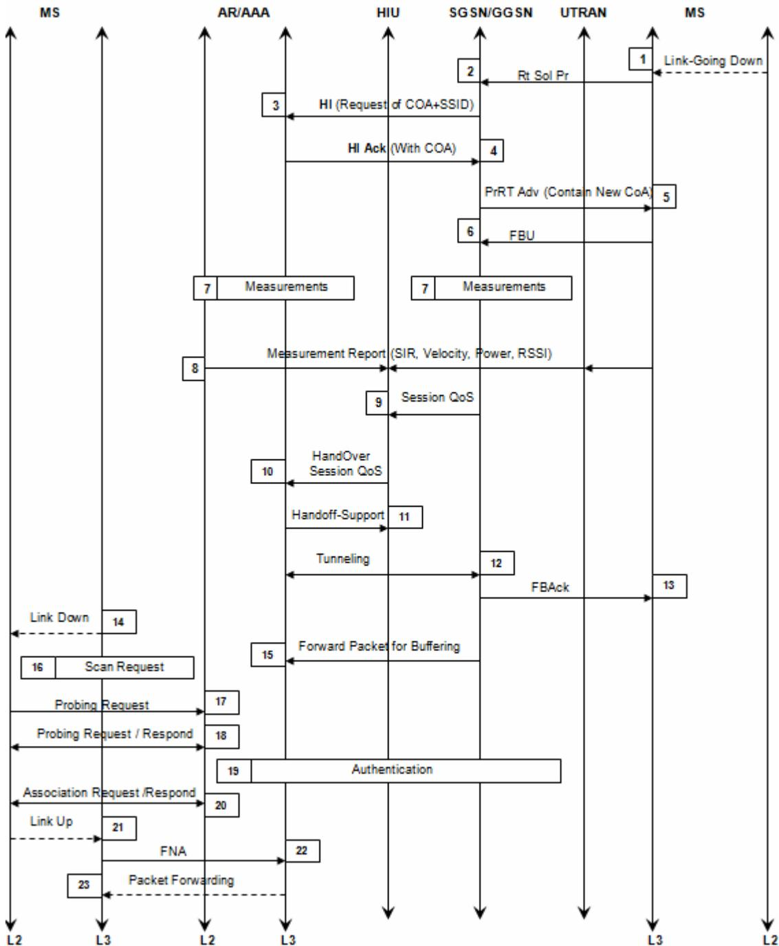
Figure 8.1.1: Handover from UMTS to WLAN Network
