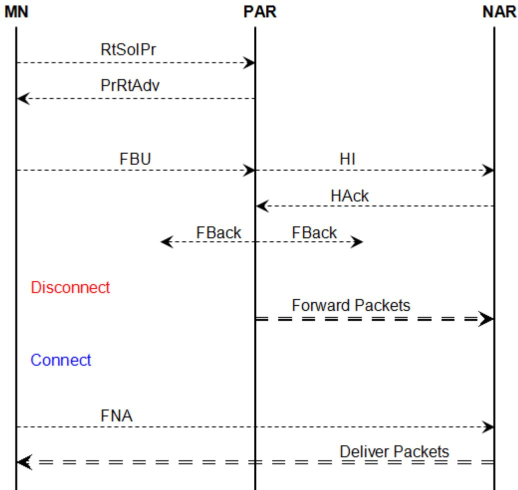
Figure 7.3.1: Predictive Mode of Fast Mobile IPv6 [18]
