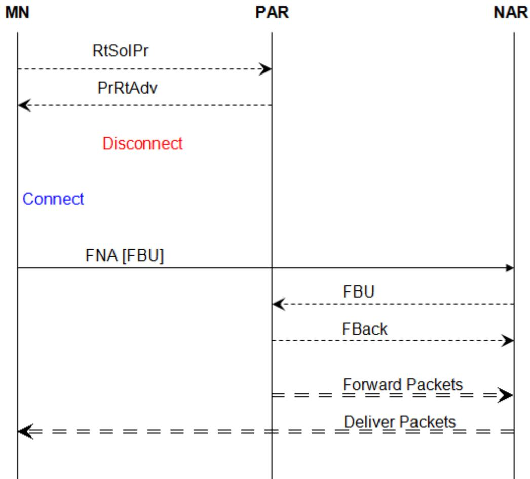
**Figure 7.3.2: Reactive Mode of Fast Mobile IPv6 [18]**
