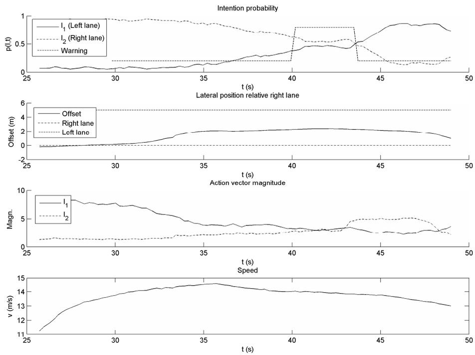
**Figure 4 - Results for manoeuvre “Between lanes”**
