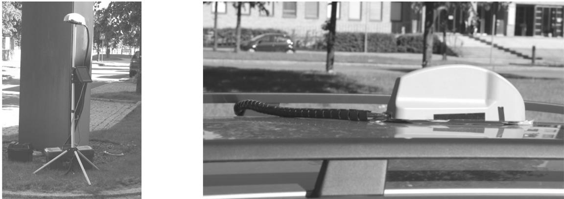
**Figure 2 - Road-side unit with HMI touch-screen (left). On-board antenna (right)**
