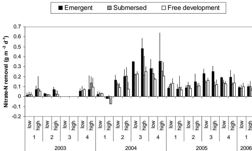
**Fig. 1.** Nitrate-N removal ( $\text{g m}^{-2} \text{d}^{-1}$ ) in wetlands containing emergent, submersed and freely developing vegetation with different hydraulic loads (low:  $0.13 \text{ m d}^{-1}$  and high:  $0.39 \text{ m d}^{-1}$ ), and during different seasons (Period 1: December to February; period 2: March to May; period 3: June to August; period 4: September to November). Error bars show standard errors.
