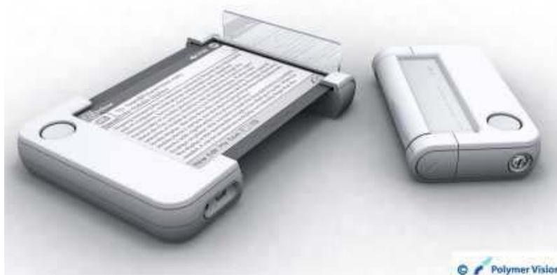
**Figure 3.** Rollable display (Source: Polymer Vision)
