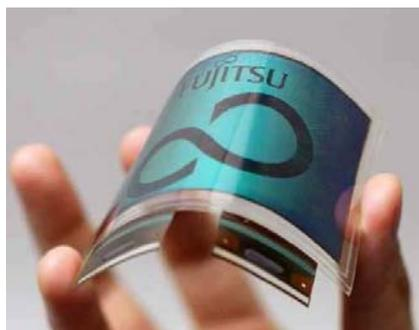
**Figure 2.** Bendable color display (Source: Fujitsu, 2006)
