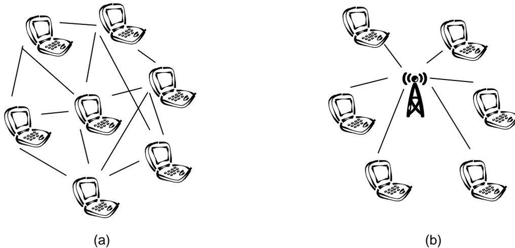
Figure 1. Two different network topologies are depicted: (a) ad hoc mode and (b) infrastructure mode.
