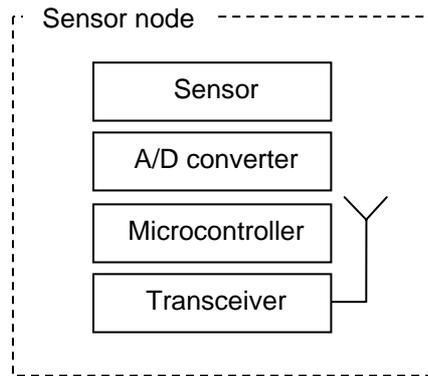
Figure 9. Schematic picture over a sensor node design.
