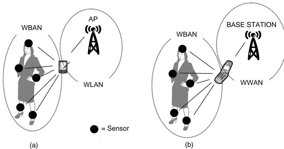
Figure 2. Two different gateways<sup>1</sup> for a WBAN: (a) WBAN connected to WLAN, (b) WBAN connected to WWAN.
