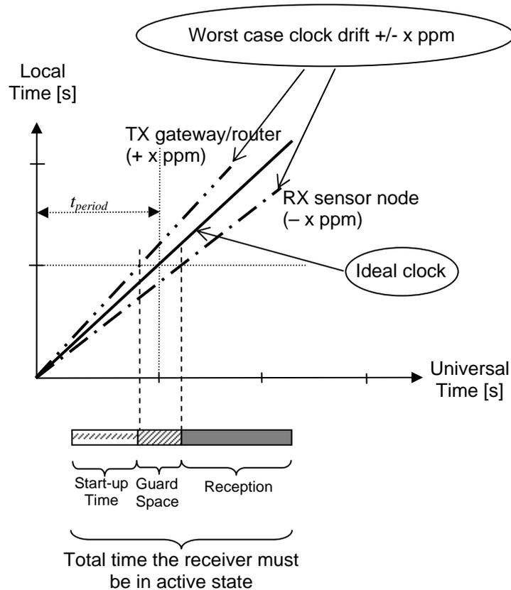
Figure 6. Clock drift at transceiver pairs, TX and RX, in sleep mode (the scale is not realistic in the graph).
