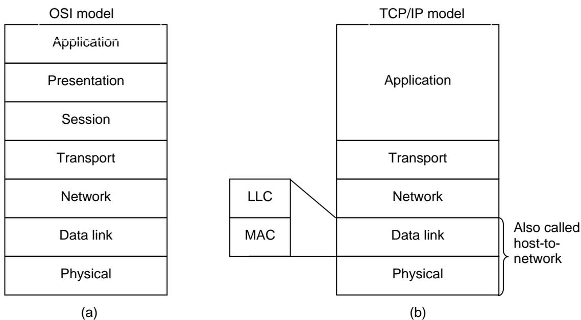
Figure 3. Two different protocol stacks: (a) OSI stack a reference model from ISO, (b) TCP/IP model used on the Internet.
