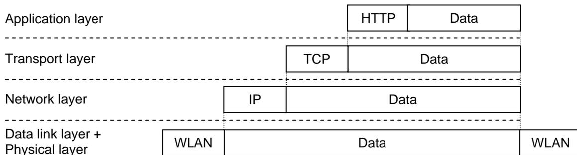
Figure 4. Packet encapsulation after a web browsing request; HTTP→TCP→IP→WLAN.
