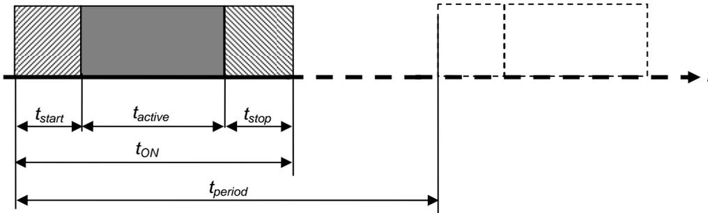
Figure 9. Duty cycling with different timing parameters.
