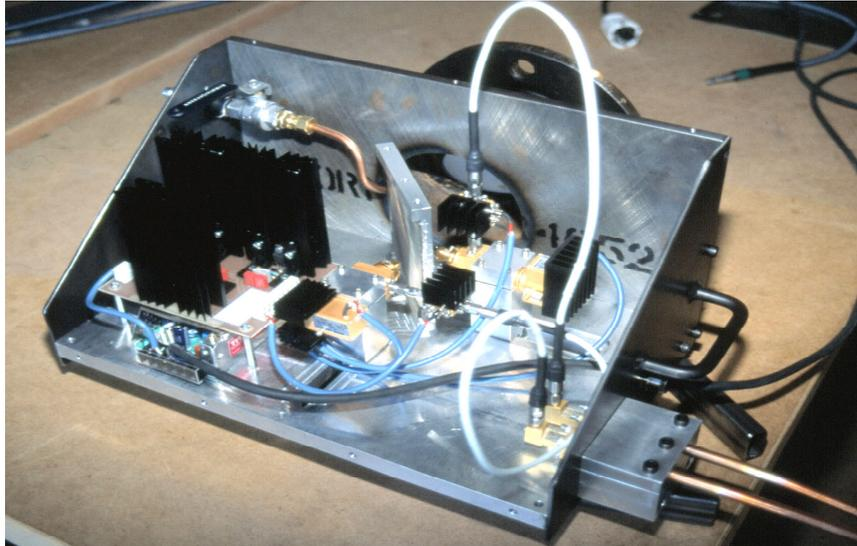
**Figure 2. Microwave Sensor Mounted in Encapsulation**
