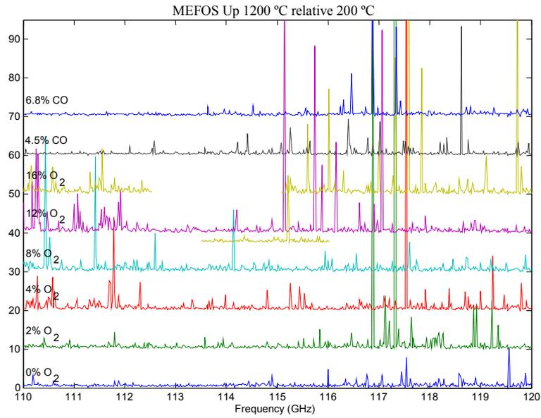
**Figure 6. Gas Spectra Received at 1200 °C for Different Molecular Mixtures**
