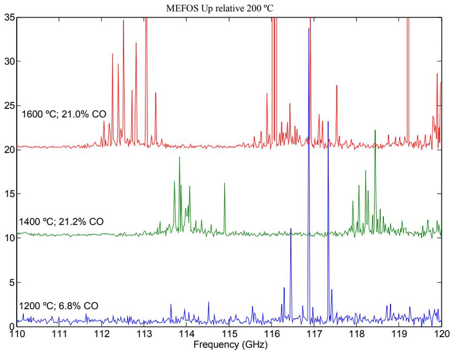
**Figure 8. Gas Spectra Received for Three Different Temperatures for CO**
