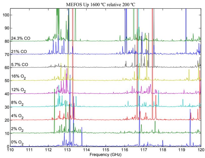
**Figure 7. Gas Spectra Received at 1600 °C for Different Molecular Mixtures**
