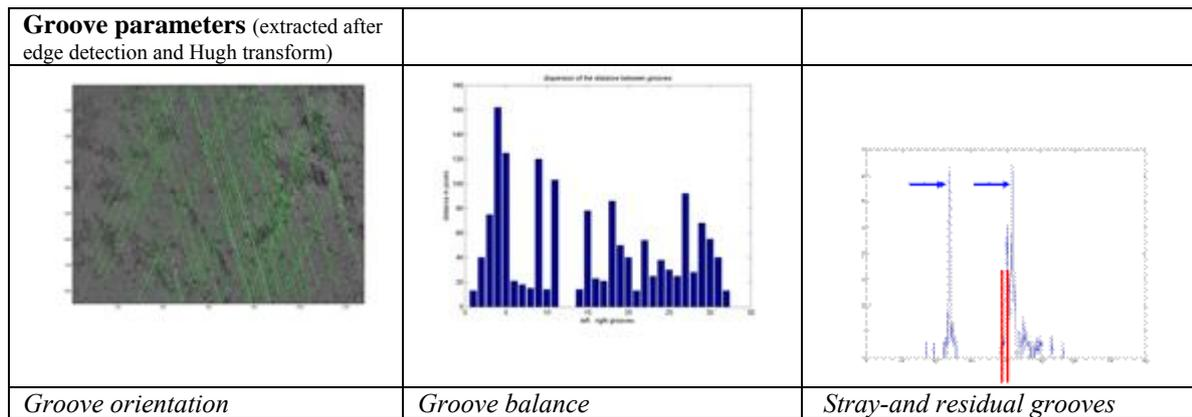
Fig. 7 After groove detection (left), groove balance (mid) and distribution of groove orientations can be calculated from the histograms. The stray- and residual grooves (right) are oriented other than the orientation of the two dominating (left-, righthand) orientations  $\theta_1$  and  $\theta_2$  in fig 5 above .
