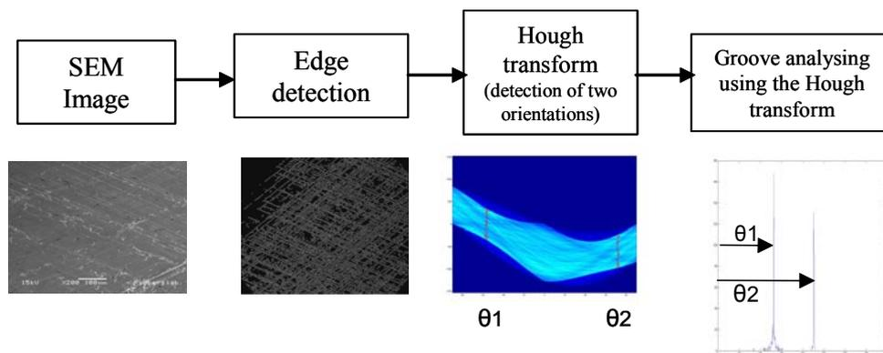
Fig. 6 By a combination of SEM imaging, classic edge detection, and analysis of the strongest parts of the Hough transform, dominant linear features as exemplified with the right most histogram at different  $\theta$ -angles
