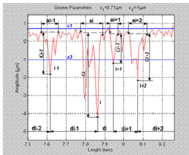
Fig. 8 Non-ISO standardized 2D profile parameters completing the SEM image analysis with groove characteristics. The three groove parameters here are; mean groove width (a), mean groove height(c) and mean distance between grooves (d).
