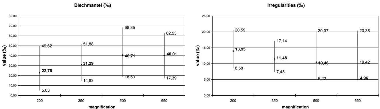
Fig. 10 Blechmantel- and irregularities parameters show a negligible sensitivity to magnification level in the SEM. Any magnification from 200X to 650X are possible to use for the analysis.
