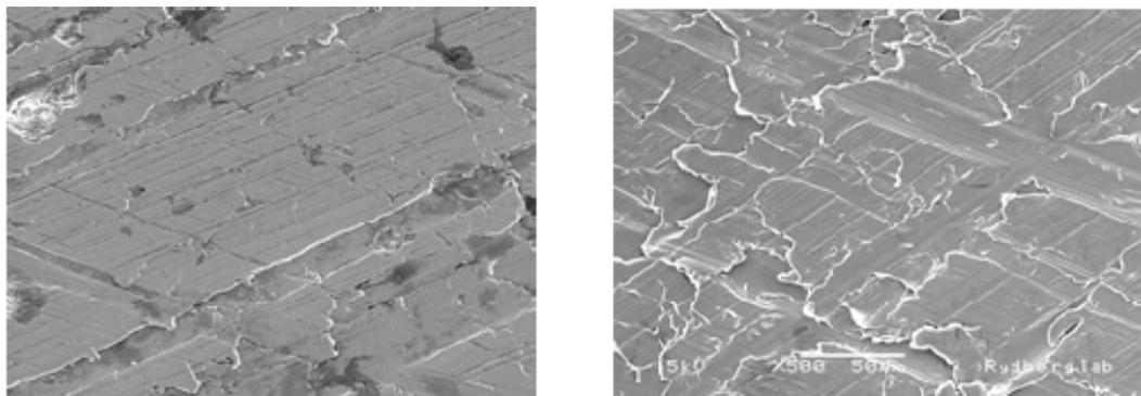
*Fig. 1 SEM pictures of two cylinder liner surfaces with different degree of folded material, so called “blechmantel”.*
