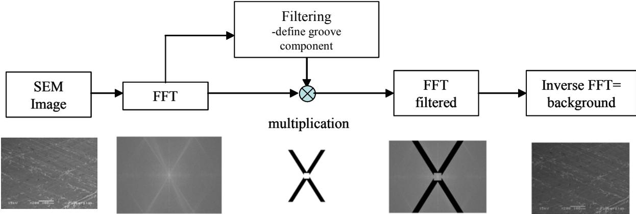
Fig. 4 The different steps followed for extracting the parameters blechmantel, irregularities and holes .
