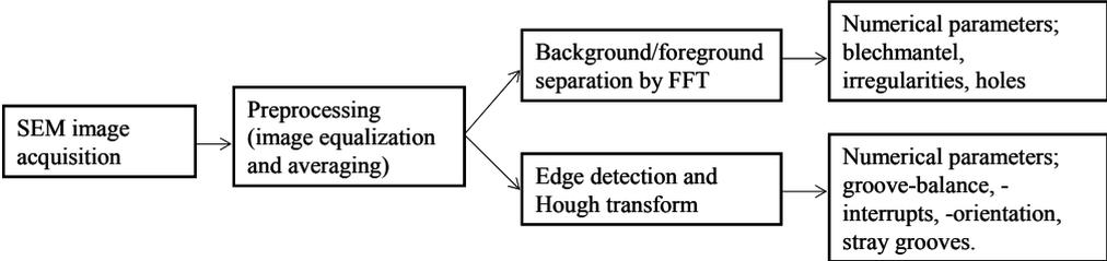
Fig.3. Workplan for the image analysis method
