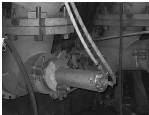
Fig. 4. The microwave unit installed on the BF.
