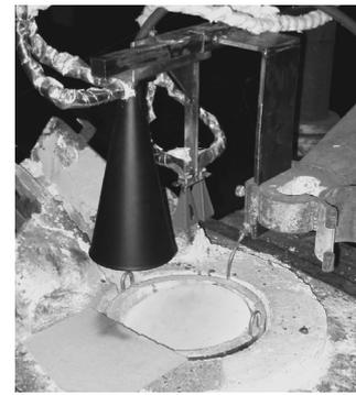
**Fig. 2.** Experimental set up with two different sets of antennas suspended above the furnace.
