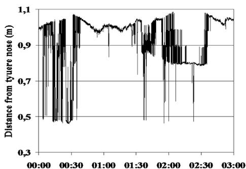
Fig. 5. Raceway depth measurements.
