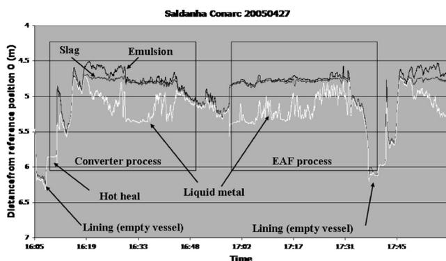
Fig. 13. Process progress (with the courtesy of Saldanha Steel SA).
