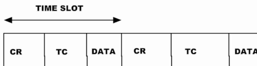
**Fig:- 29 Frame Format (redrawn from [50])**
