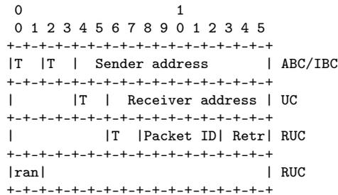
Figure 3.9: Bit-oriented Rime packet header generated by IPS (no alignment required).
