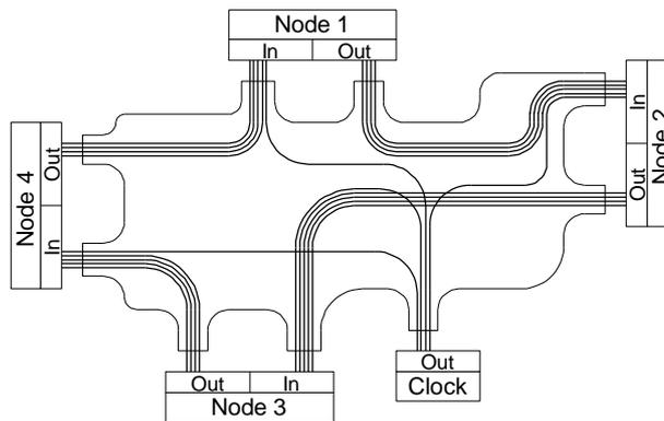
Figure 15: A foil of fibres connects four computational nodes. In addition, a clock node distributes clock signals to the computational nodes.
