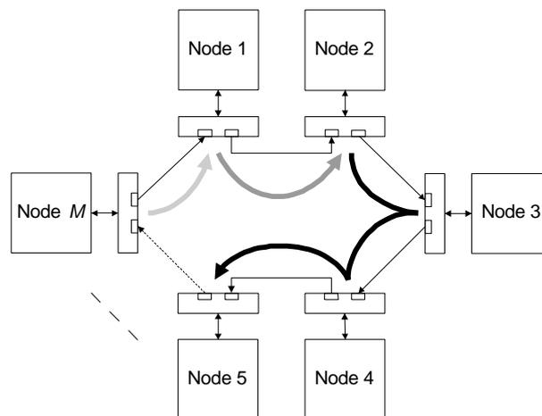
Figure 13: Example of spatial bandwidth reuse. Node M sends to Node 1 at the same time as Node 1 sends to Node 2 and Node 2 sends a multicast packet to Nodes 3, 4, and 5.
