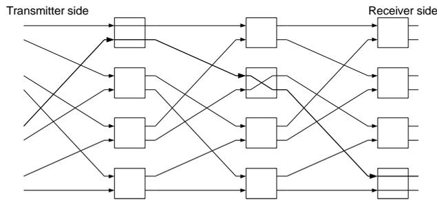
Figure 4: Omega network for an eight-node system. One path through the network is highlighted.
