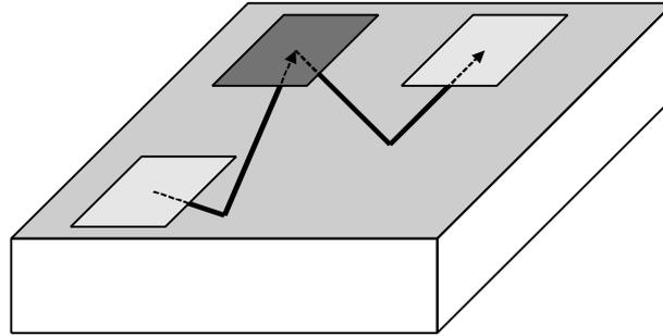
Figure 17: Example of a planar free space system. The direction of the beam is steered by the optical element on the way between two chips.
