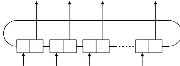
Figure 12: Ring network as switch-fabric.
