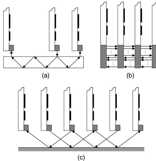
Figure 18: Optical backplane configurations: (a) with planar free space optics, (b) with smart pixel arrays, and (c) with a mirror.
