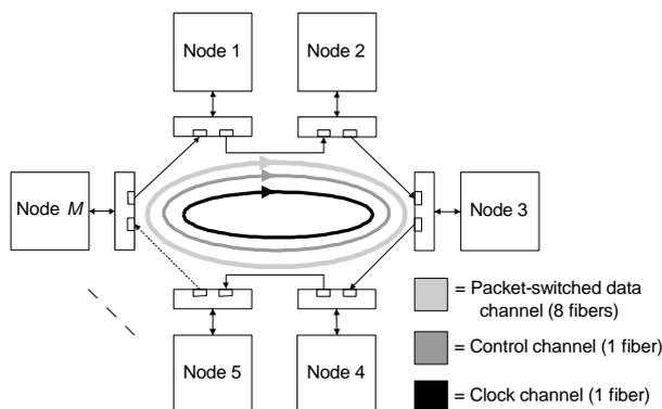
Figure 14: Control channel based network built up with fibre-ribbon point-to-point links.
