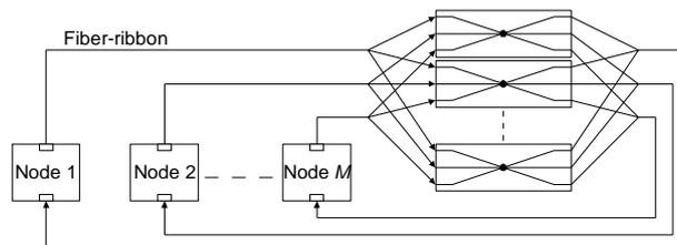
Figure 16: Array of passive optical stars connects a number of nodes via fibre-ribbon cables.
