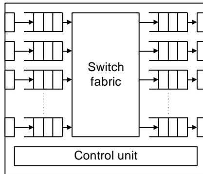
Figure 2: An example of switch architecture.
