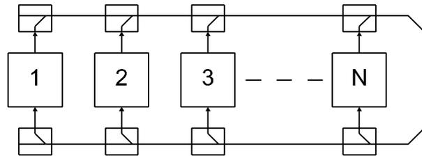
Figure 8: Folded fibre-optic bus.
