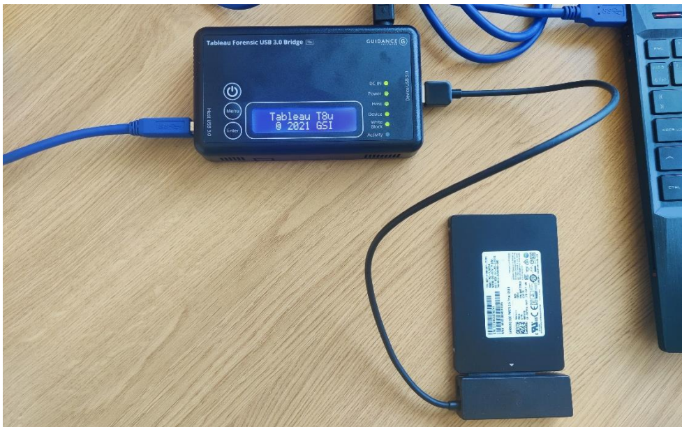
Figure 2 – Picture of the write blocker and disk 1
