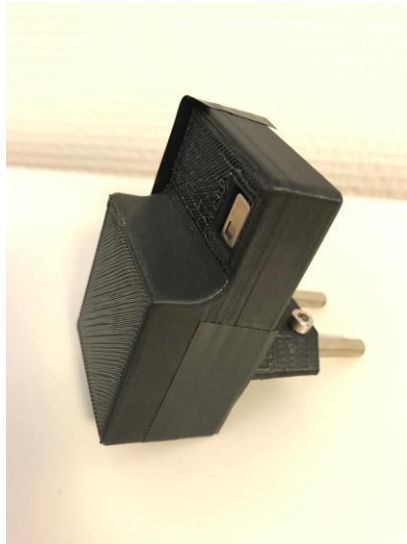
Figure 1. A prototype of Griddy with the Panasonic Grid-EYE infrared thermopile array sensor visible on the front.
