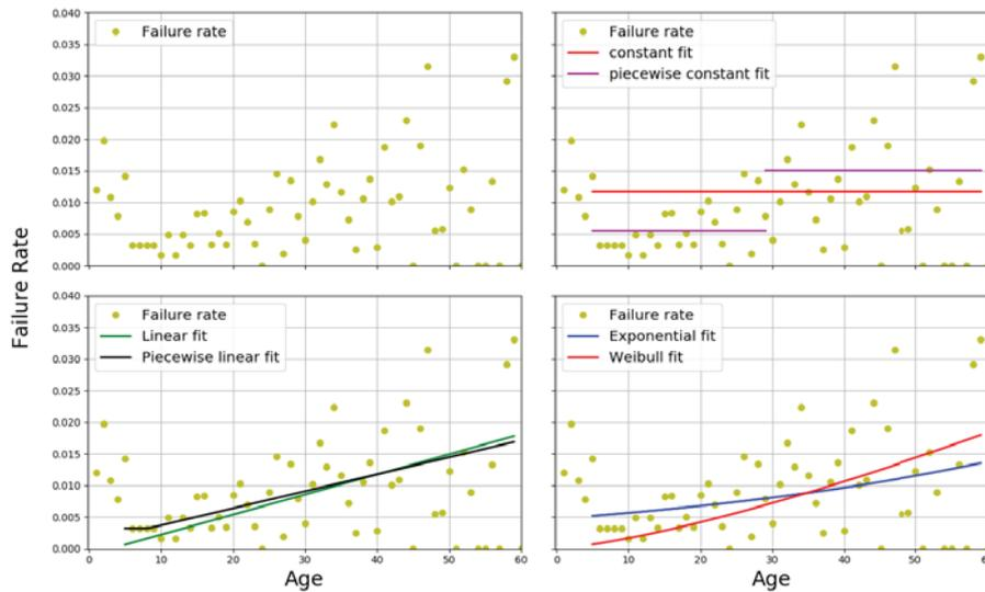
**Figure 3.8:** Six different failure rate models, fitted to the empirical data after removing the incorrect failures.
