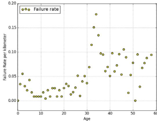
**Figure 3.7:** Empirical failure rate per kilometer as function of age, for high voltage PILC cables.
