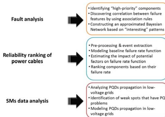
**Figure 3.1:** The procedure of the proposed data-driven method for weak spot detection in SDGs.
