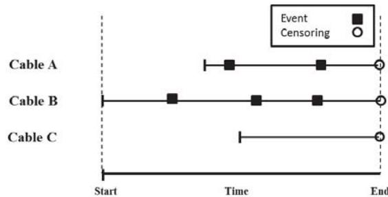
**Figure 2.3:** Schematic plot for events and censoring in feeder lines.
