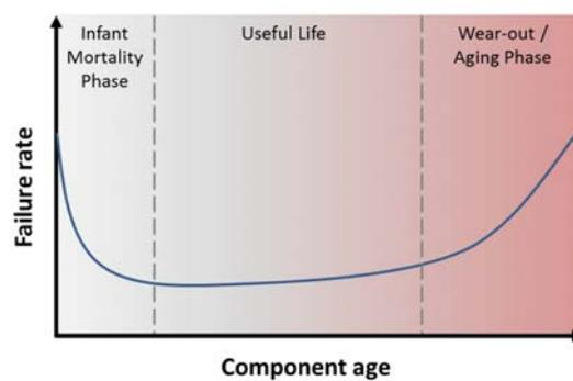
**Figure 2.1:** Bathtub curve of typical failure rate for components.
