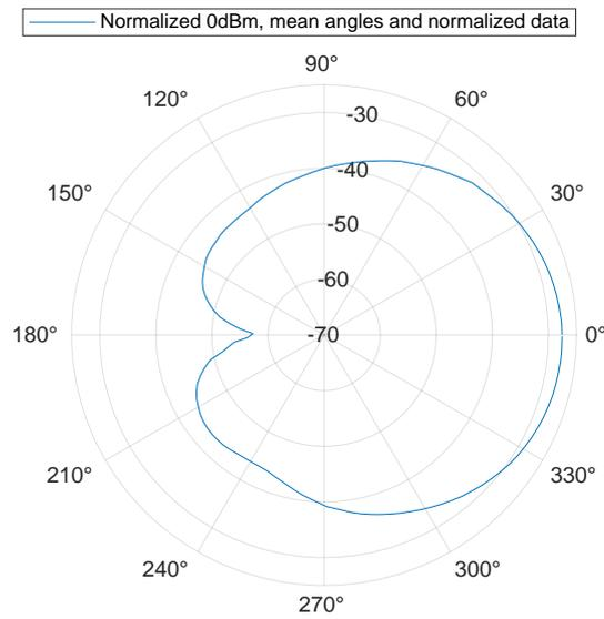
Figure 26: Graphs of measured data at 0dBm that has been plotted. a) is the horizontal radiation pattern and b) is the vertical radiation pattern. c) is the norm data with angles that are the mean of vertical and horizontal.
