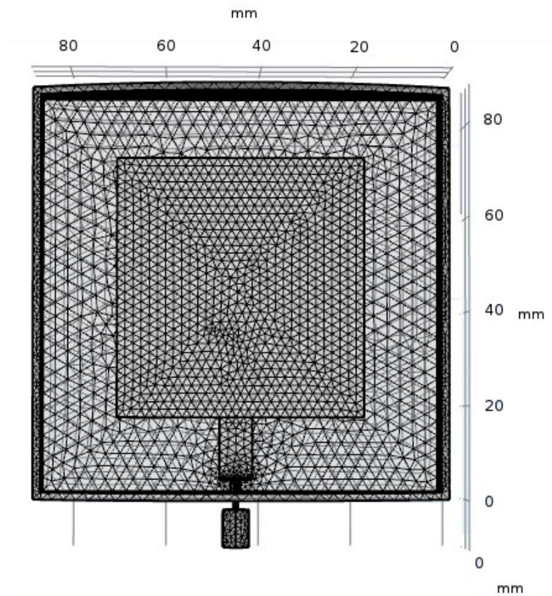
Figure 12: simulated vertical Patch antenna with mesh from comsol
