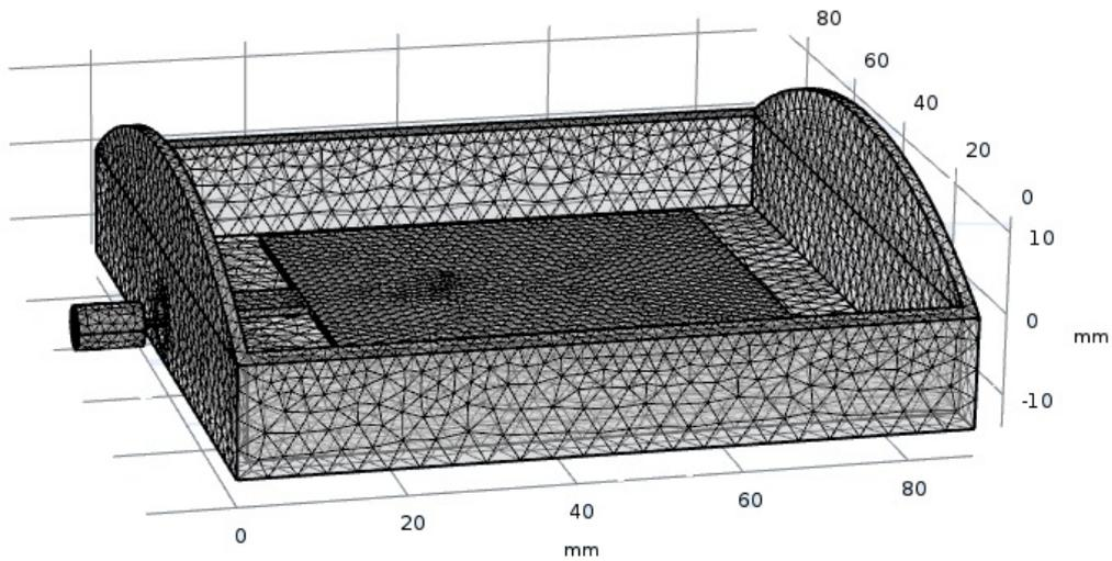
Figure 11: simulated horizontal Patch antenna with mesh from comsol
