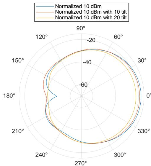
(c) Vector norm of the radiation pattern in 10dBm, 10dBm with 10tilt and 10dBm with 20tilt
