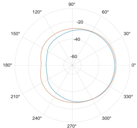
(b) The blue polar plot indicates a 10dBm 20tilt measured polar plot and the red polar plot indicates a 28dBm 20tilt simulated polar plot.
