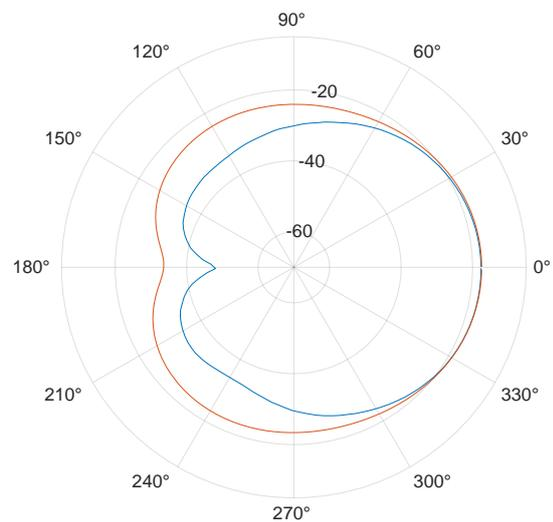
(b) The blue polar plot indicates a 10dBm measured vector norm polar plot and the red polar plot indicates a 32dBm simulated polar plot.
