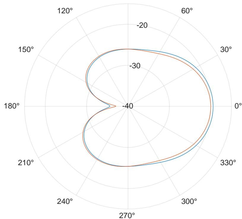
Figure 2: The norm of the E field that is obtained from figure 1. The blue polarplot is 30 dBm, the red polarplot is 30dBm with 5 deg tilt
