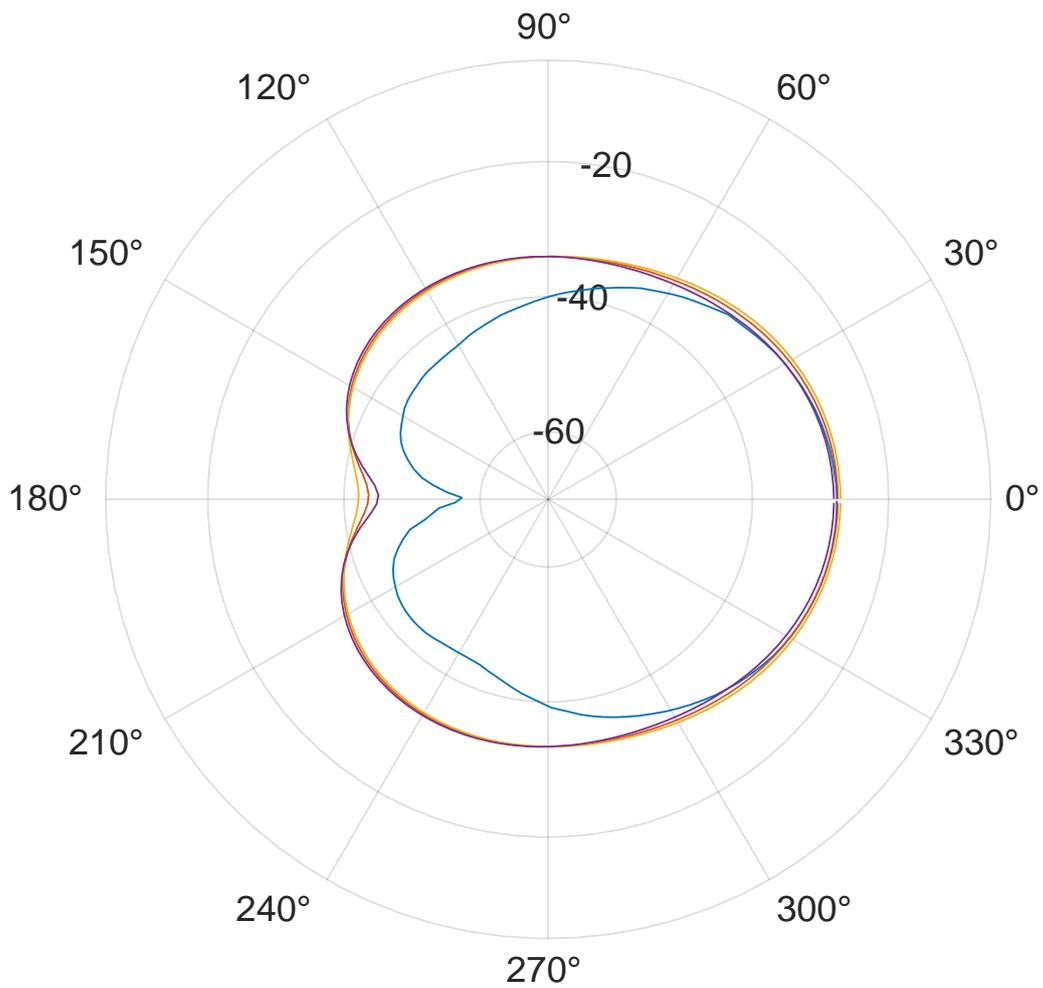
Figure 20: A 3D simulated 22 dBm polar plot compared to a 0 dBm measured data polar plot. The blue polar plot is the measured at 0dBm at 0 degrees. The red polar plot is the simulated at 22dBm at 0°. The yellow is the simulated at 22dBm with a negative tilt of 5°. The purple is the simulated at 22dBm with a positive tilt of 5°.
