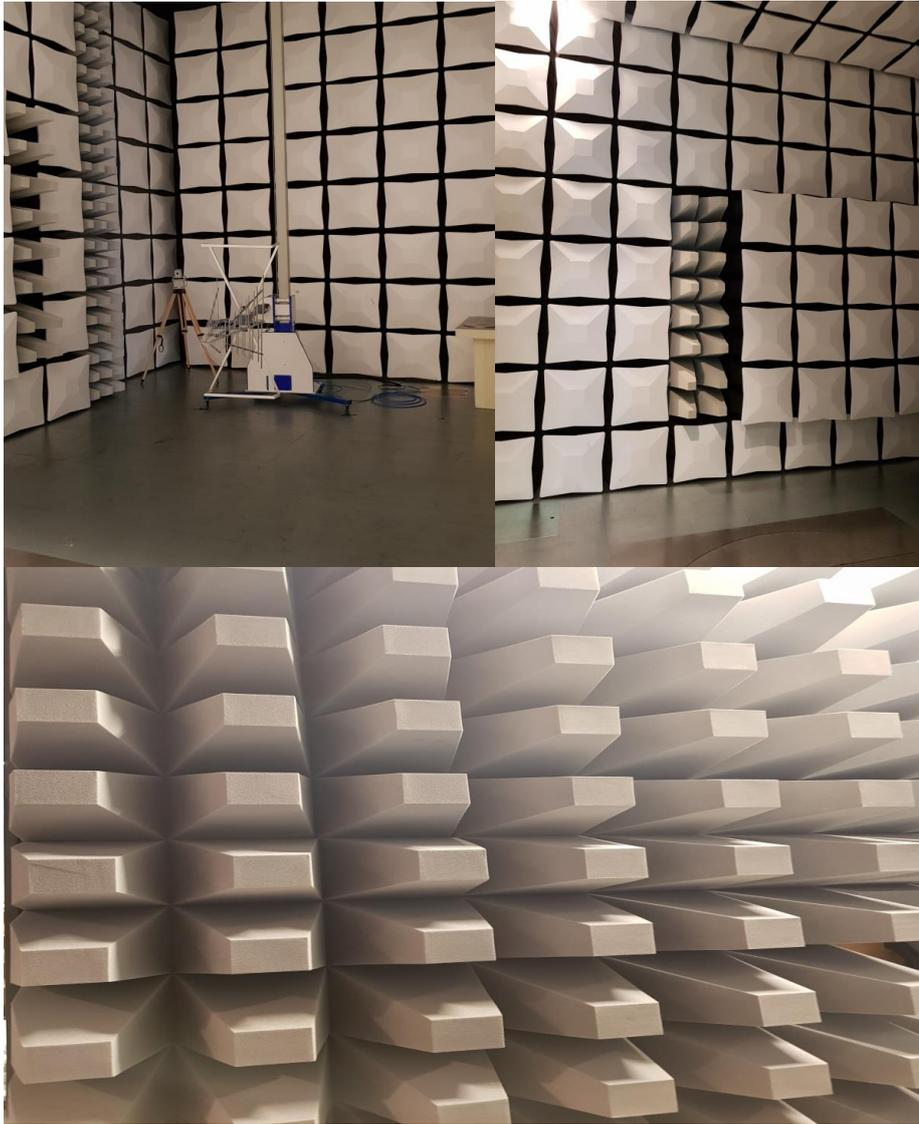
Figure 7: An anechoic chamber located in Halmstad university. A receiving antenna which is usually connected to a signal generator is shown. EM-absorbent foam is placed around the room to minimize EM-radiation being reflected.
