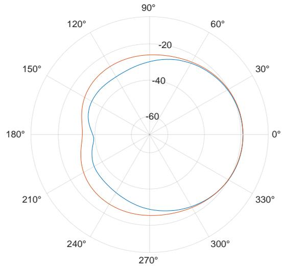
(b) The blue polar plot indicates a 10dBm 10tilt measured polar plot and the red polar plot indicates a 30dBm 10tilt simulated polar plot.
