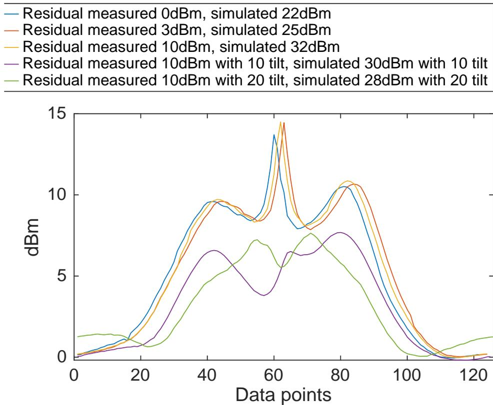
Figure 17: In this figure all residuals have been plotted together. This is done to be able to spot similarities and differences. The residuals have between 122-126 data point. Every data point is an difference between simulated data and measured data at an specific angle.
