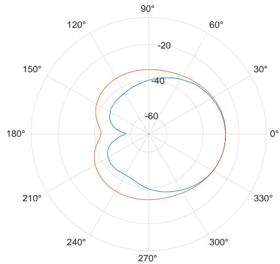
(b) The blue polar plot indicates a 0dBm measured vector norm polar plot and the red polar plot indicates a 22dBm simulated polar plot.
