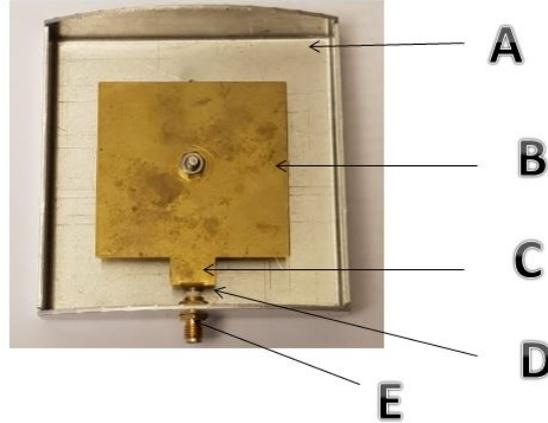
Figure 10: Patch antenna
