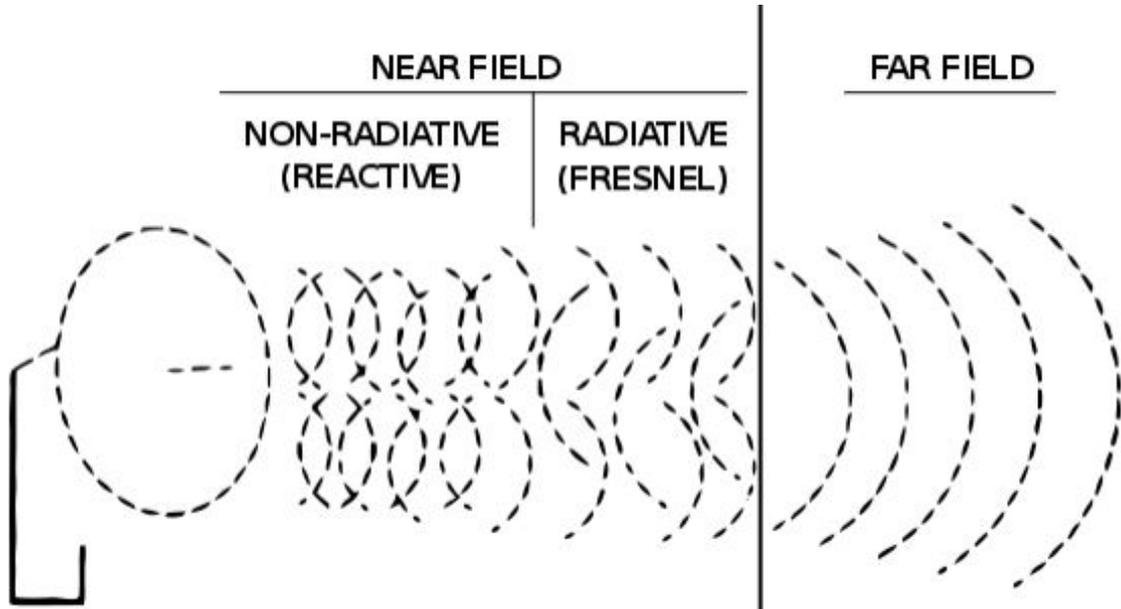
Figure 3: Differences between Fresnel diffraction in the near field area and Fraunhofer diffraction in the far field area
