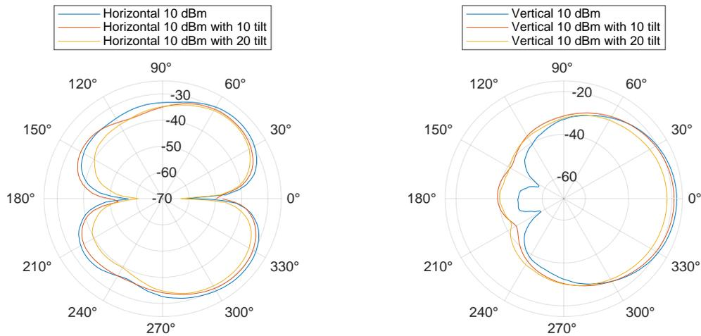
(a) Horizontal radiation pattern 10dBm, 10dBm with 10tilt and 10dBm with 20tilt
