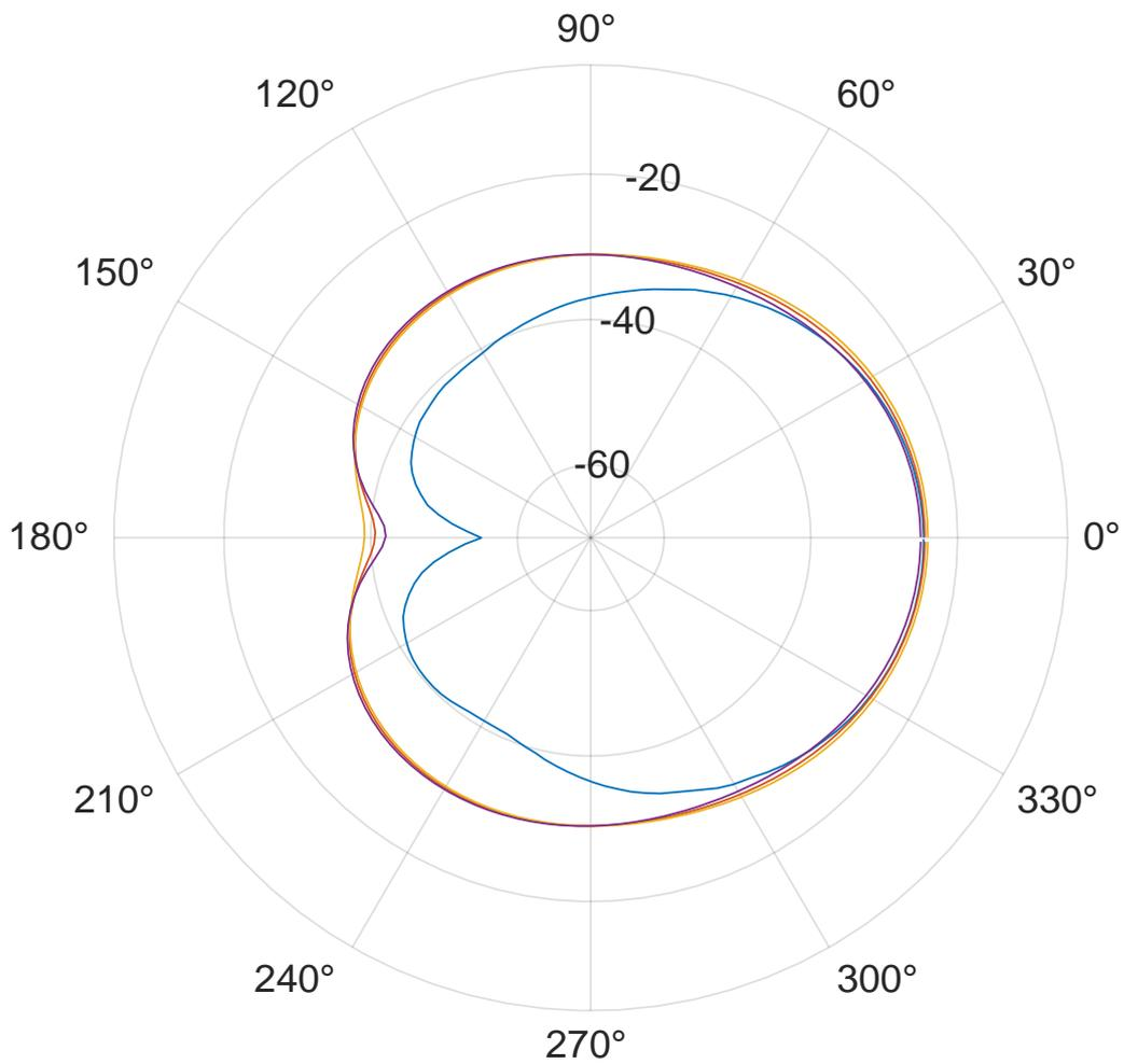
Figure 21: A 3D simulated 25 dBm polar plot compared to a 3 dBm measured data polar plot. The blue polar plot is the measured at 3dBm at 0 degrees. The red polar plot is the simulated at 25dBm at 0°. The yellow is the simulated at 25dBm with a negative tilt of 5°. The purple is the simulated at 25dBm with a positive tilt of 5°
