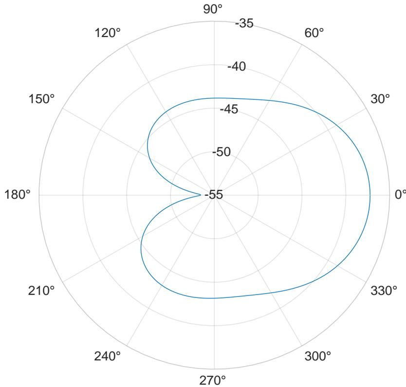
Figure 4: A vertical polar plot representation of a simulation of an antennas radiation pattern. Radial scale in dBi.
