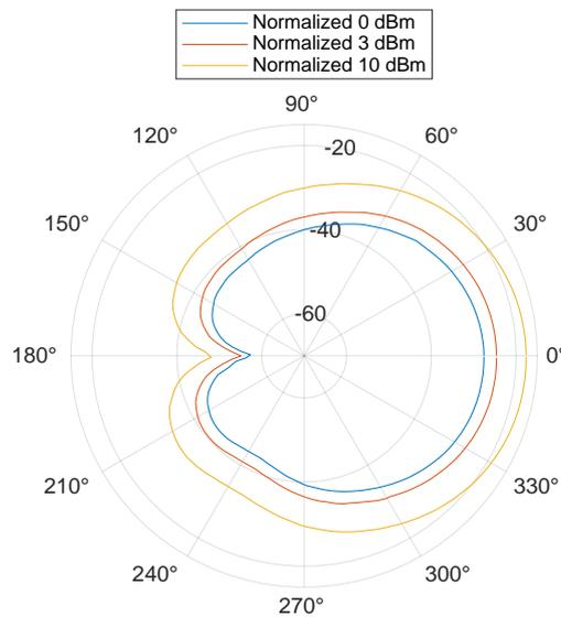
(c) Vector norm of the radiation pattern in 0dBm, 3dBm and 10dBm
