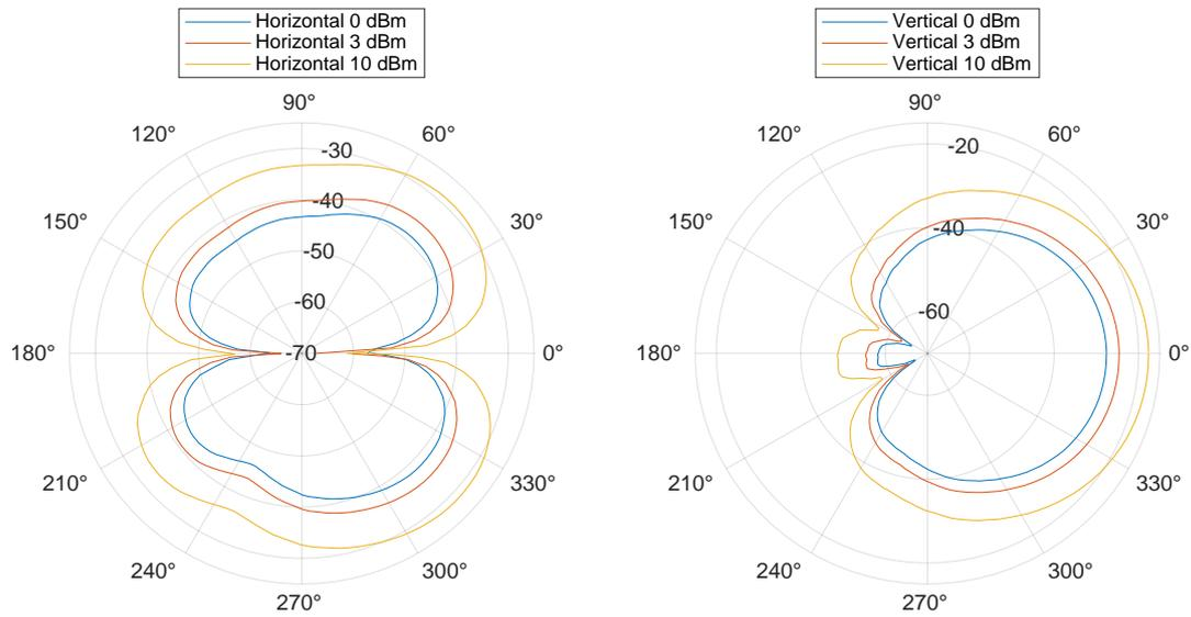
(a) Horizontal radiation pattern from 0dBm, 3dBm and 10dBm
