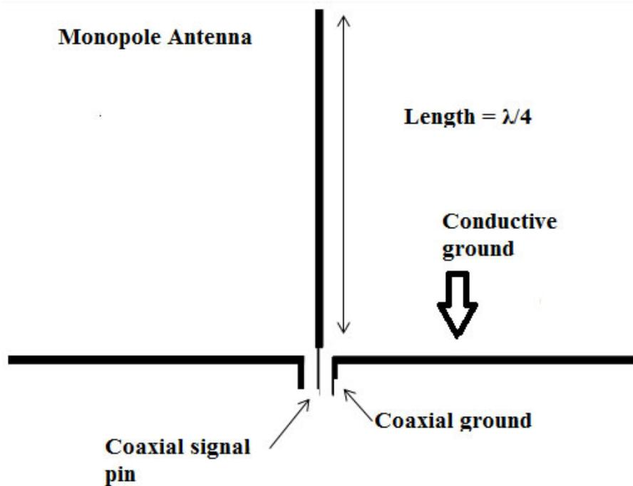
Figure 5: Dimensions of the monopole antenna
