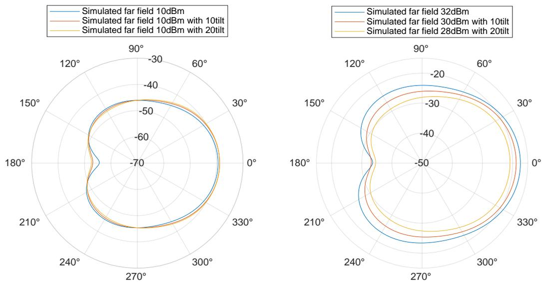
(a) Graphs of simulated data at dBm values 10,10 with 10tilt and 10 with 20tilt.
