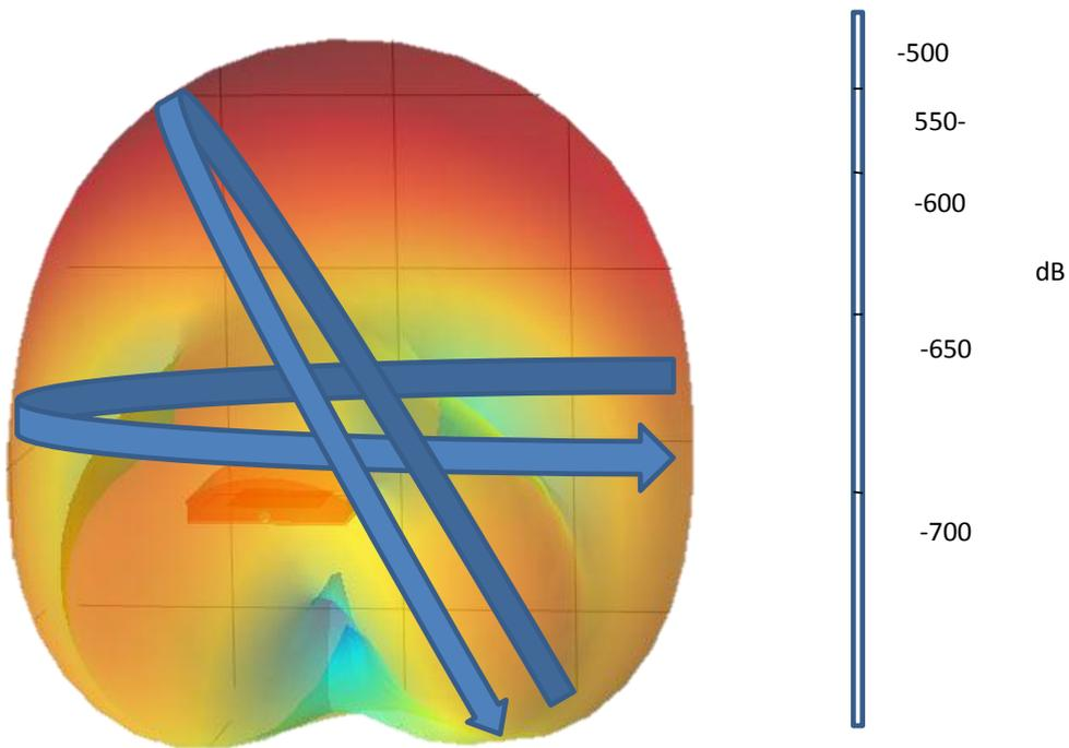
Figure 1: A 3d simulation of a patch antenna's radiation pattern. The arrow pointing downwards indicates a tilted vertical plane while the arrow pointing towards the right indicates the horizontal plane. The scale is in dB.
