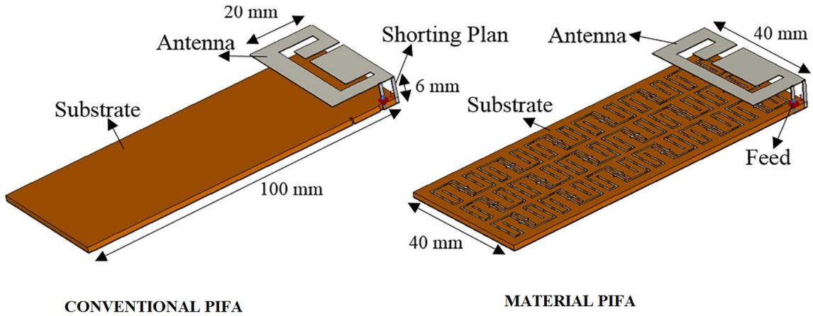
Figure 6: On the left is the geometry of the conventional PIFA and on the right is the metamaterial- embedded PIFA for cellular phones [17]
